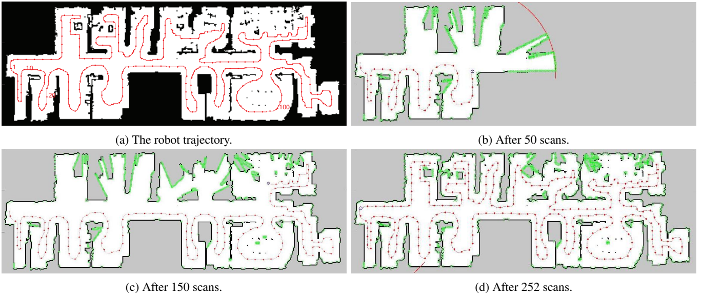
Figure 2: The Freiburg environment (Trajectory 1), 414 \times 149 cells. a) Lines show the robot trajectory, and the dots show the poses where scans were taken and frontiers evaluated. b, c, d) The robot is shown with a small blue circle, frontiers are marked with green crosses, and a red arc shows the robot’s FOV.
