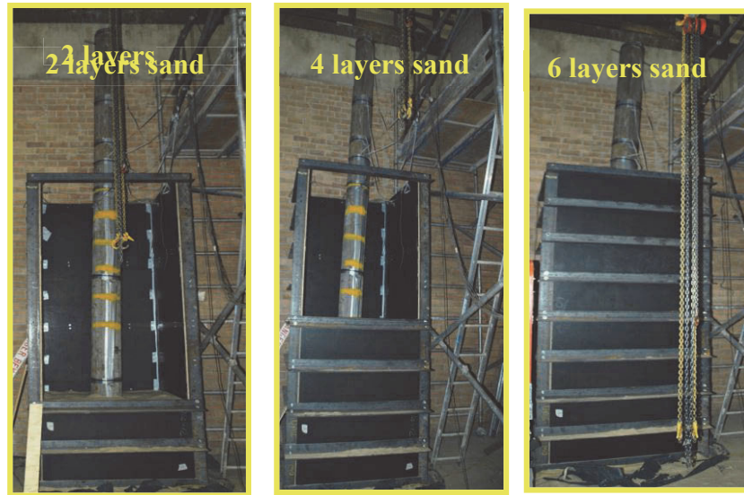
Figure 4.16 The laboratory set-up for NDT methods under embedded conditions for a timber pole
