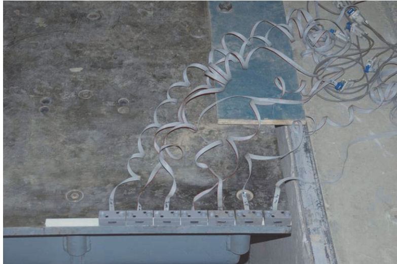
Figure 4.5 Calibration of the accelerometers using a shake table
