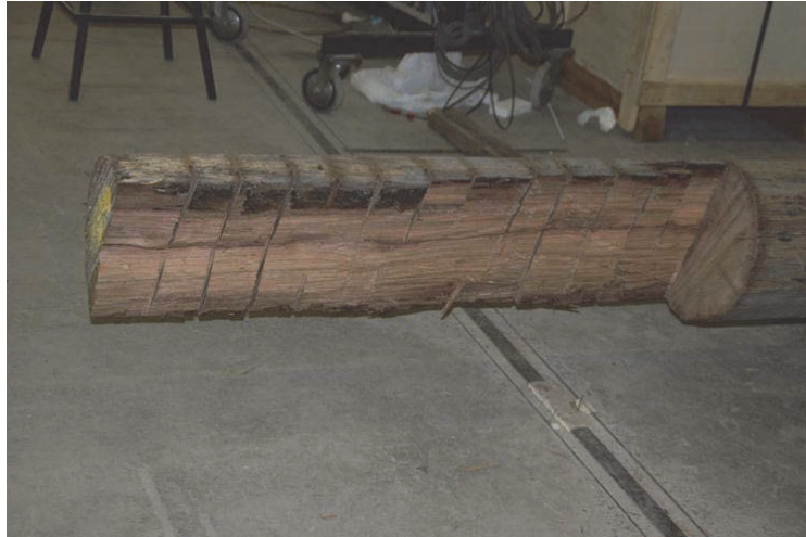
Figure 4.18 side view of a typical damage inflicted in timber pole in laboratory
