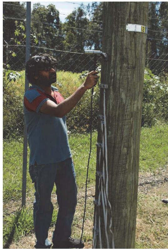
Figure 4.26 Schematic and photo of test set-up of embedded BW tests for field testing.
