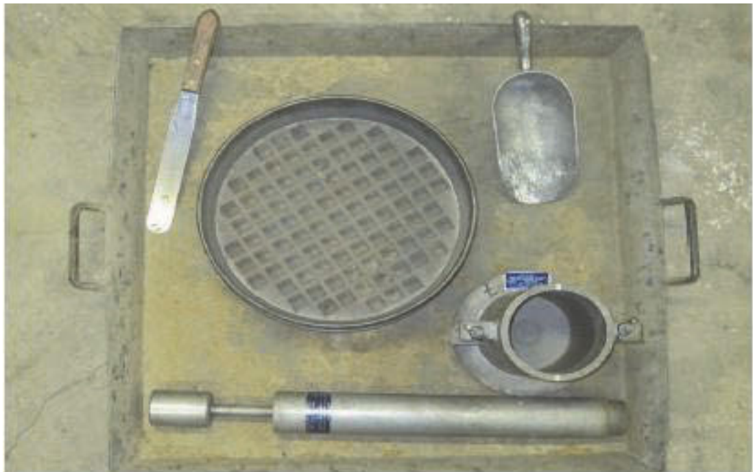
Figure 4.32 Compaction test equipment
