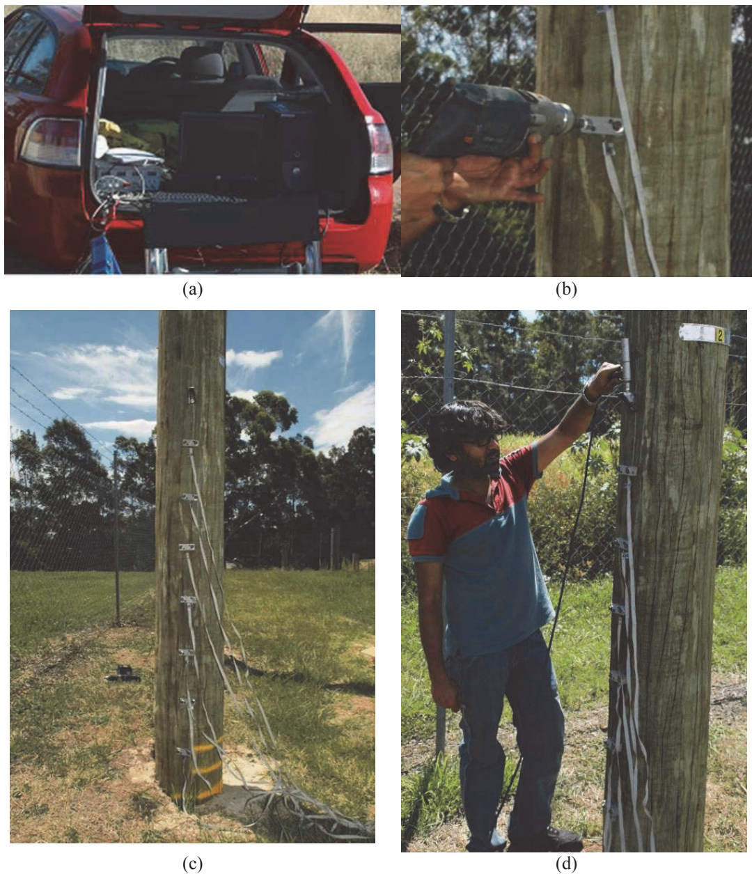
Figure 4.10 Testing procedure: (a) setting up of equipment, (b) mounting of accelerometer, (c) attached bracket and accelerometers and (d) execution of the test.
