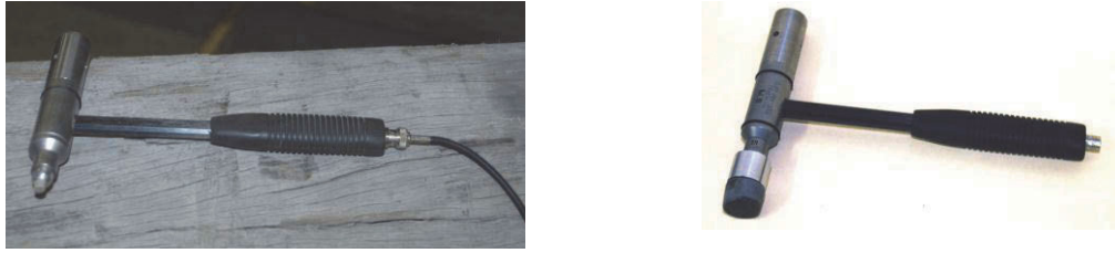
(a) (b) Figure 4.1 Impact hammer (a) stiff tip, (b) soft tip
