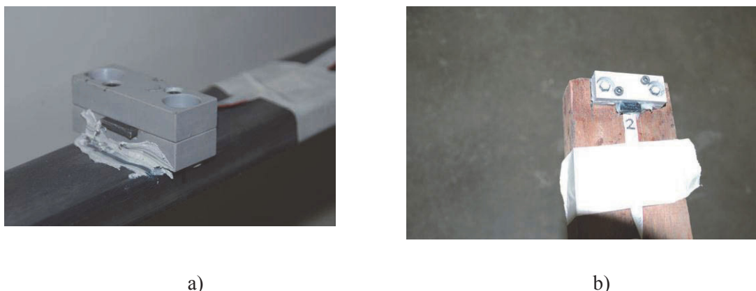
Figure 4.4 Accelerometers mounted to the a) steel beam and b) timber beam by screws
