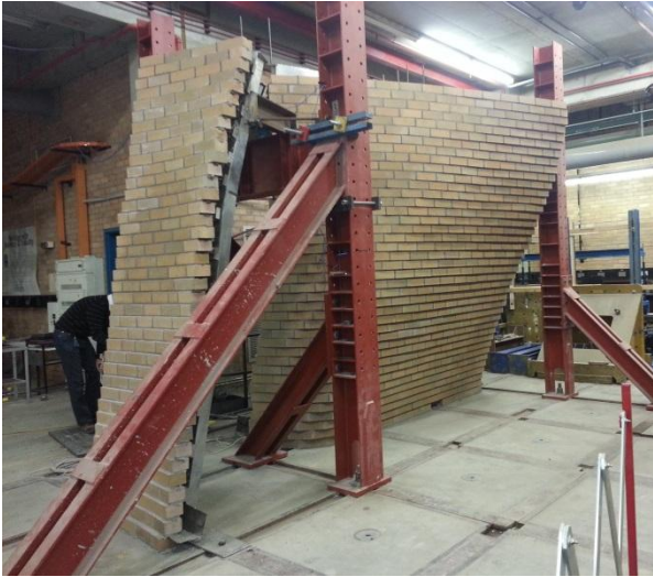
Figure 10: Completed mock-up panels. Leaning-in panel (Left) and leaning-out panel (right)
