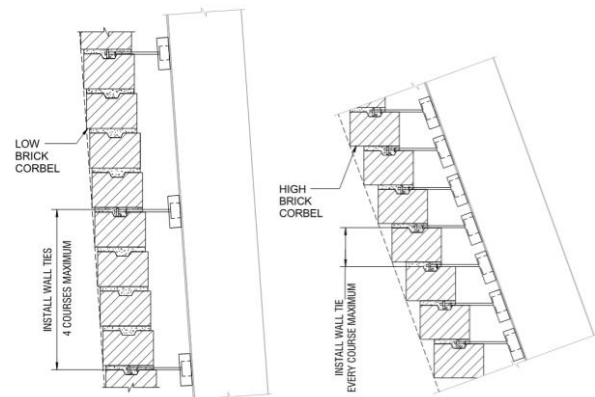
Figure 20: Wall sections showing tie arrangement for a near vertical wall (left) and heavily corbelled wall (right)
