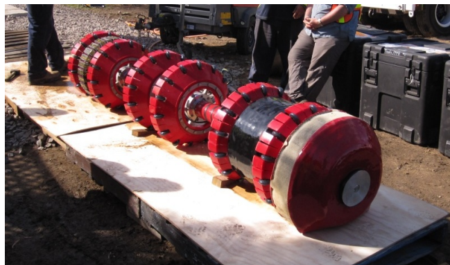
Figure 1: Russell NDE Systems Inc. Sea-Snake in-line tool used to detect pipeline corrosion, pitting, wall thinning and graphitisation.
