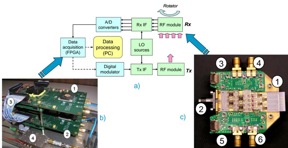
Figure 1: a) System block diagram; b) Photograph of the digitizer module assembly where 1 and 2 are two identical digitizers, 3 is interconnect cable and 4 is a sampling oscillator; c) Photograph of the RF module assembly where: 1 is the antenna array; 2 is the LO input; 3-6 are IF outputs.
