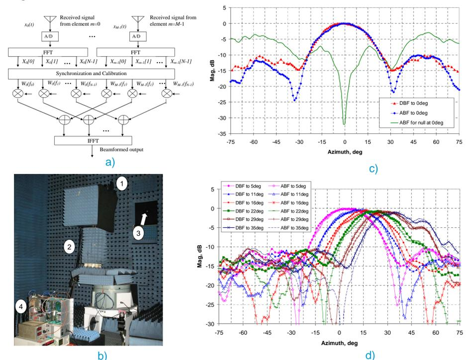
Figure 2: a) Structure of the DBF; b) System test setup in the 12m far field anechoic chamber where 1 is the receive array RF module, 2 is the rotator and 3 is the transmit antenna aperture, 4 are the modulator, IF module, digitiser & power supplies; c) Measured E-plane co-polar DBF and ABF array patterns at 0° azimuth; d) Measured E-plane co-polar DBF and ABF array radiation patterns for a selection of positive azimuth angles.
