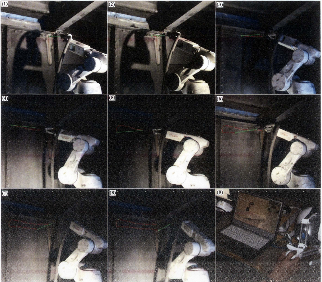
Figure 4.33 Snapshots of the field test: the manipulator performs a dry run sandblasting
