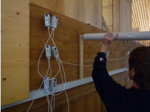
Figure 10 Sensors attached to glulam beams to detect delaminations and to estimate MOE.
