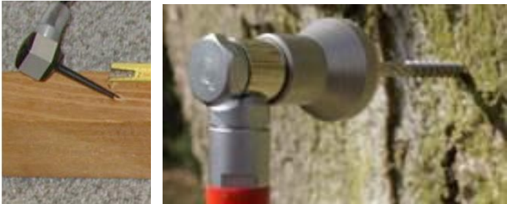
Figure 3 Accelerometer attachments with (a) a spike [9] and (b) a screw connection (IML GmbH).
