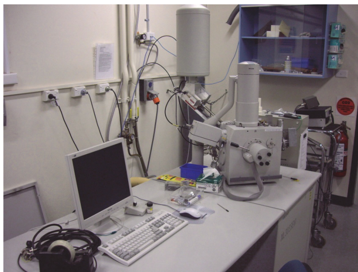
Figure 3.0: The XL30 ESEM with original PDS prior to modifications and upgrades.
