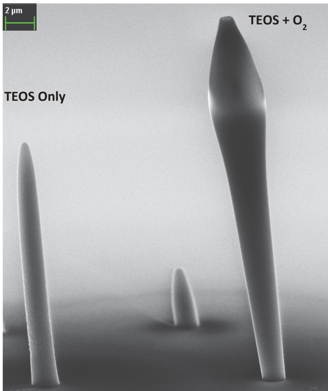
Figure 6.7: Two FEBID pillars (set 5) grown under identical conditions excepting the addition of 0.24 torr of O 2 for the pillar on the right. TEOS partial pressure was 0.05 torr.
