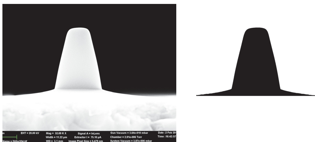
Figure 3.16: (Left): High contrast & resolution image for volumetric analysis. (Right): The image on the left is converted to a binary image where only the pixels of the deposit are black. The co-ordinates of the black pixels are exported as a text-file for input to the volumetric estimation program
