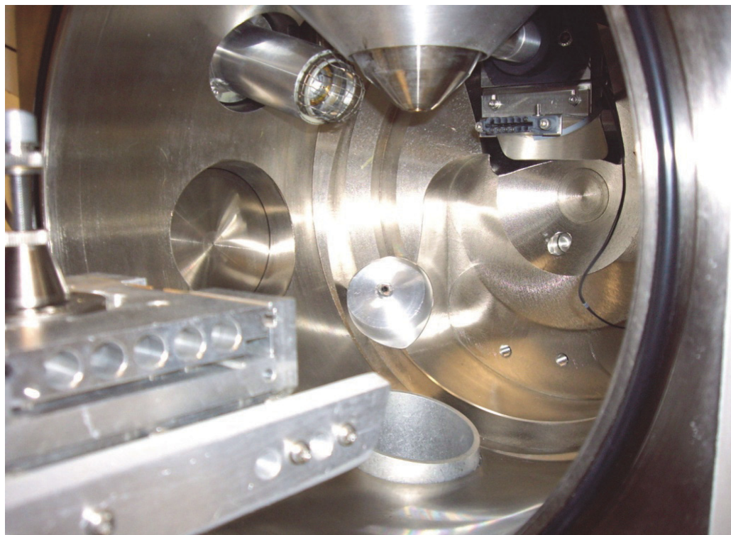
Figure 3.3: Photograph of the interior of the XL30 ESEM specimen chamber. Many O-ring seals are present and they may add to precursor gas contamination by diffusion of atmosphere into chamber through O-rings.
