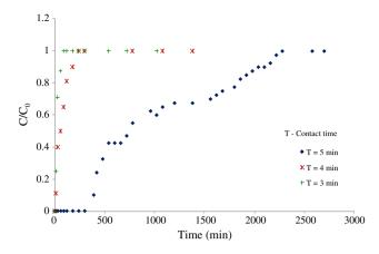
Fig. 5. Breakthrough curves for recycled water softening process with different contact times
