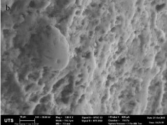
Fig. 3. SEM images of the raw natural zeolite (a) and after pre-conditioning (b).
