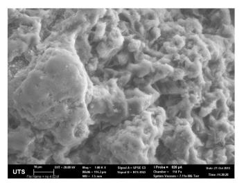
Fig. 4. SEM image of the zeolite after the column reached saturation.
