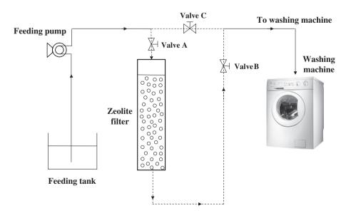
Fig. 1. Schematic diagram of the pre-treatment unit.
