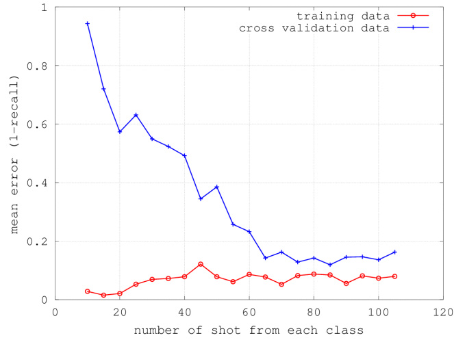
Figure 5.4.1: Training dataset size selection by analysing the classification performance on different dataset size from each shot class. For this experiment k = 10 and n = 5 are used.
