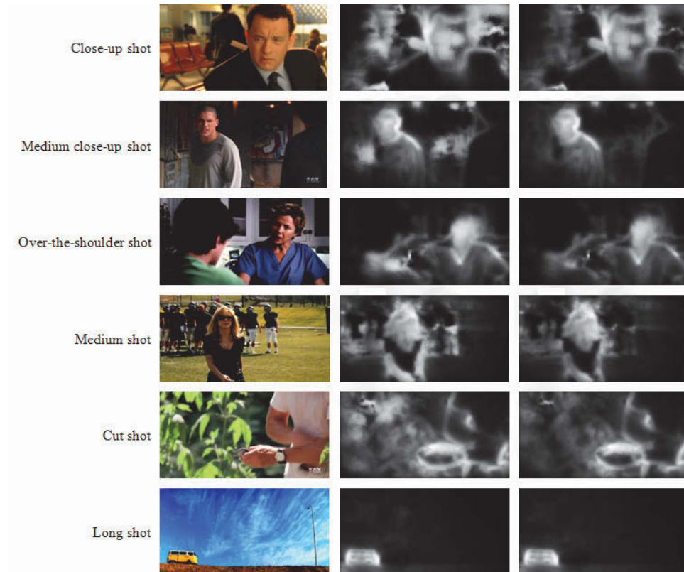
Figure 3.3.2: Examples of most commonly appeared shot types in movies, corresponding contrast saliency maps (third column from left) and context saliency maps (right column) using proposed method.
