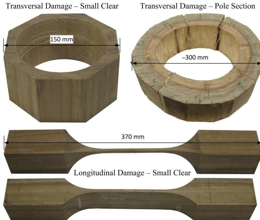
Figure 6-6: Small clear specimens and cross-sectional pole sections used for damage detection
