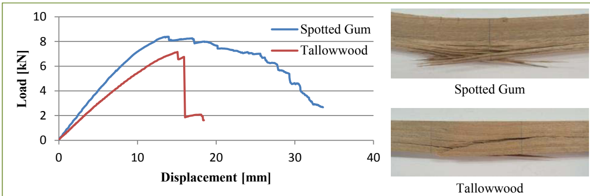
Figure 4-7: Comparison of the typical failure behaviour (curves) and failure mode (pictures) of Spotted Gum and Tallowwood for the 4-point bending tests
