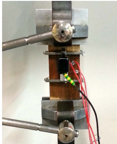
Figure 4-6: Test setup for the Poisson's ratio measurements
