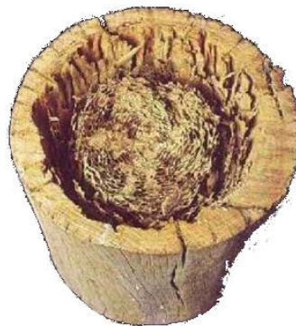
Figure 2-8: Subterranean termite nest in below ground portion of hardwood pole (Forest Research Institute NZ 1976)
