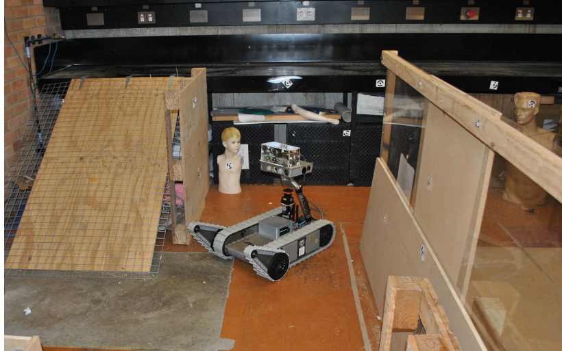
Figure 3.1: The rescue robot on the mock-up urban search and rescue test arena.
