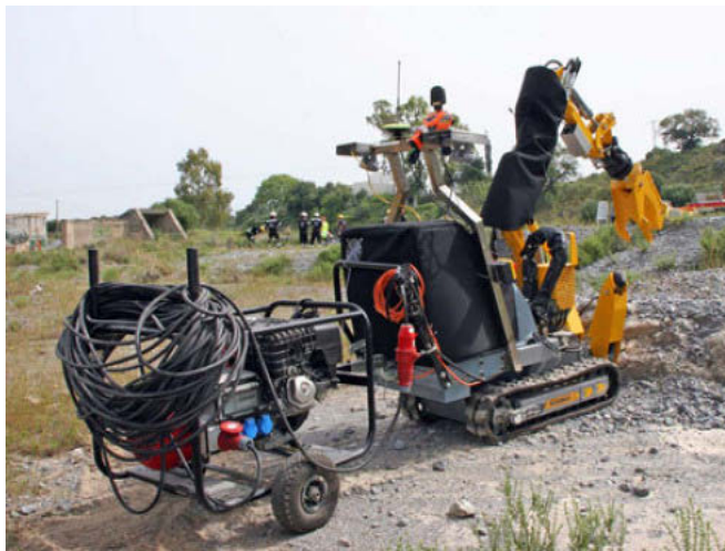
Figure 2.3: Tracked mobile manipulator Alacrane (right) and its trailer (left) during an emergency response exercise [27].
