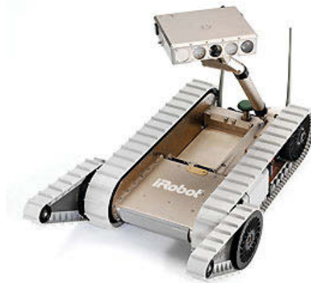
Figure 2.17: The basic model of Packbot robot without additional sensors and processing units [39].
