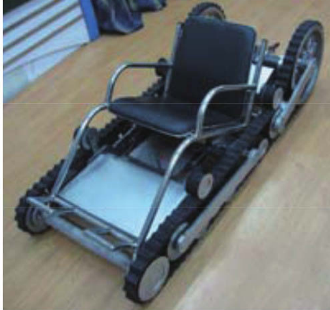
Figure 3.7: The reconfigurable tracked wheelchair robot [8].
