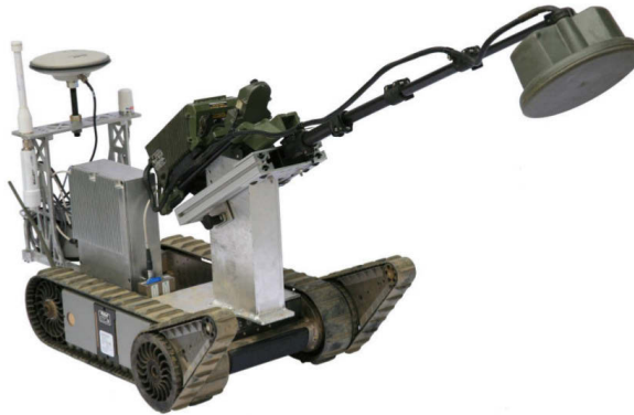
Figure 2.4: A photograph of the modified Packbot Fido from iRobot used in tip-over validation tests [16].
