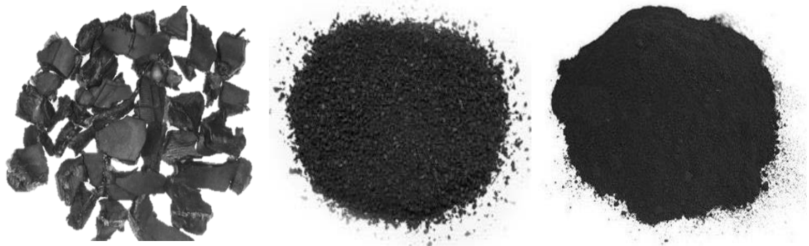
Figure 2.2: Main types of recycled rubber used in cementitious products (a) chipped rubber, (b) crumb rubber and (c) ash rubber
