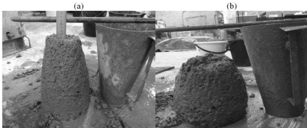
Figure 4.2: WC =0.45 (a) adjusted to the slump of 60 \pm 10 mm, (b) addition more WR caused a higher slump up to 100 mm without segregation, shear or collapse slump
