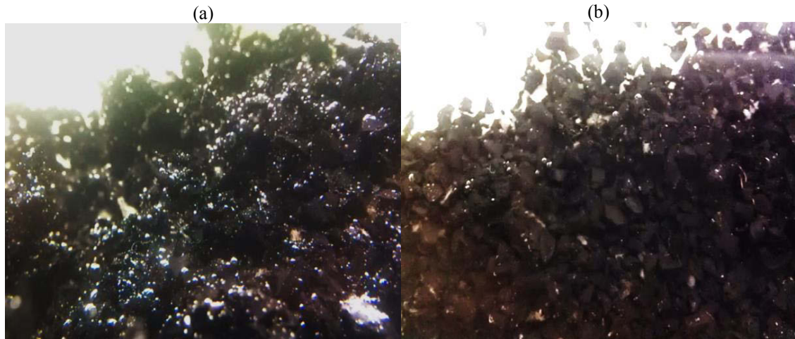
Figure 4.5: Effect of soaking rubber (a) instantly mix of rubber and water is full of air bubbles, (b) after 24 hours most of the air bubbles were released from the mix
