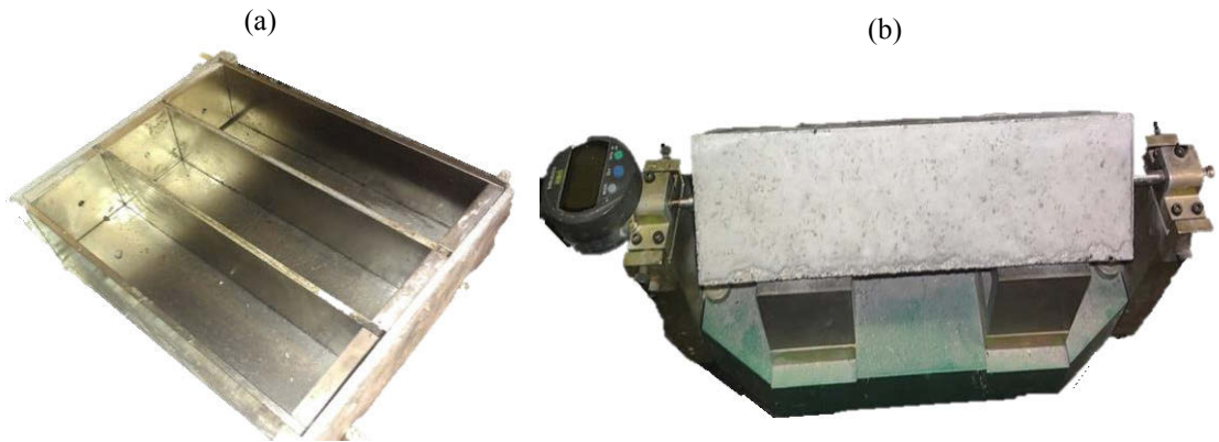
Figure 3.14: Drying shrinkage (AS 1012.13) setting, (a) moulds and (b) measurement setting
