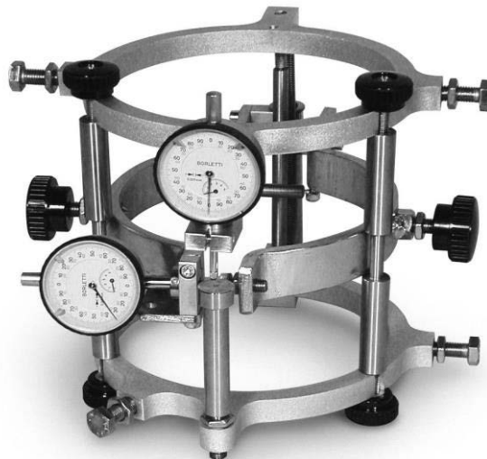
Figure 3.10: The compressometer arrangement for measuring the longitudinal strain
