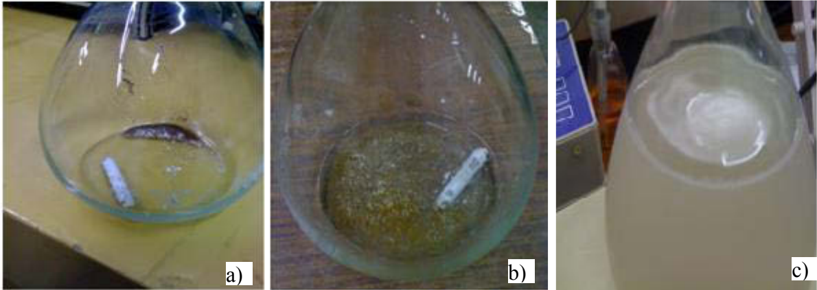
Fig. 4.2 Impurities observed during DS preparation from various commercial fertilizers a) \text{NH}_4\text{Cl} b) MAP and c) KCl
