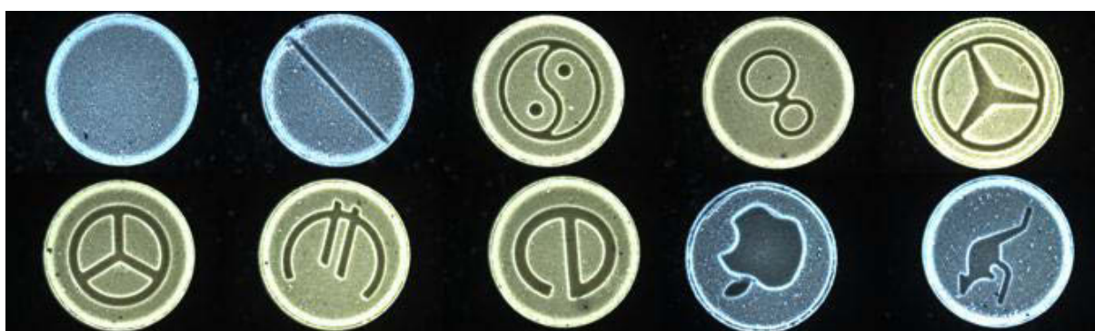
Figure 3.12: Examples of images taken with the ring light lowered towards the tablets. Row 1: “blank”, “score”, “Yin and Yang”, “8-ball” and “three-pointed star 1”; Row 2: “three-pointed star 2”, “Euro”, “e”, “apple” and “kangaroo”.
