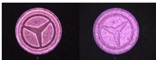
Figure 4.1: An example of a pair of images of the same tablet under different lighting conditions. The left-handed image is used for logo extraction, while the right hand image is used to extract other features.
