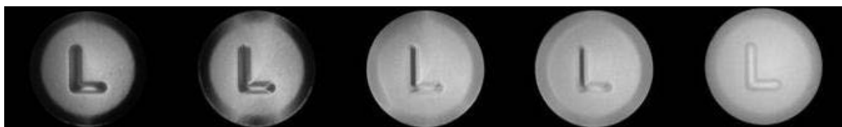
Figure 3.7: Left four images: Images generated by the four images as shown in Figure 3.6 using minimum, 2 nd minimum, median and average pixel greyscale values respectively; Right image: Same tablet under uniform lighting.
