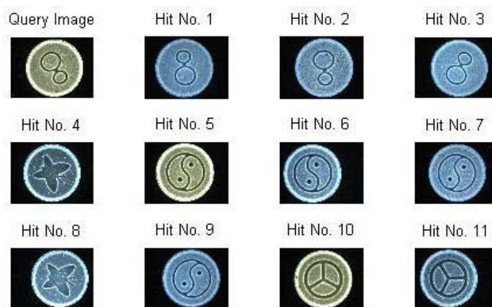
Figure 3.23: An example of a search for “8-ball” logos by Euclidean distance using Zernike moment invariants.
