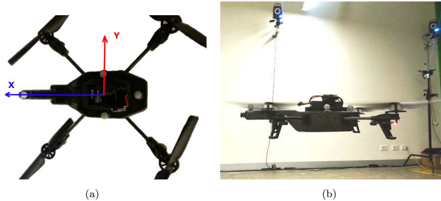
FIGURE 2.8: Vicon motion capture setup. (a) - ARDrone quadrotor attached with four reflective markers. Also shown is the body coordinate frame. (b) - ARDrone quadrotor operating in the Vicon environment. Note the Vicon IR cameras fixed to the wall.
