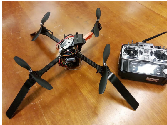
FIGURE 2.1: A typical quadrotor MAV. Shown on the side is the radio controller used for manual piloting.
