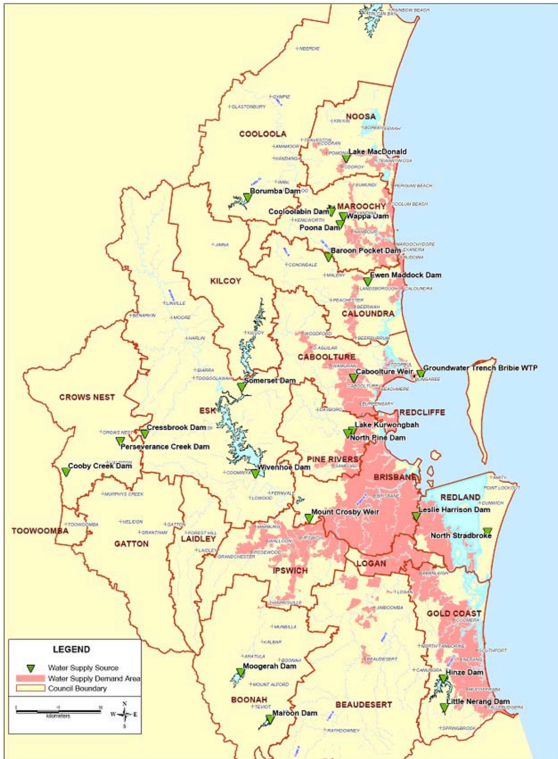
Figure 2-7 Existing water supply sources – SEQ
