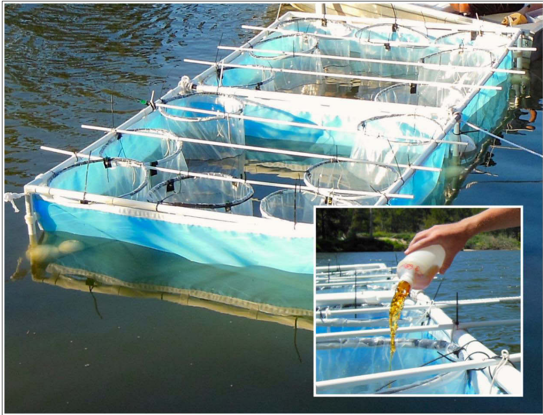
Figure 6.1. Experimental design for mesocosm experiment on the Bega River. The smaller plastic bags are the 400L mesocosm, whilst the larger outside structure protects the bags from damage. Inset adding DOC leachate at day 0.
