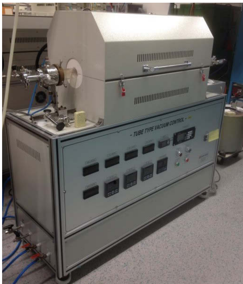
Figure 2-3 The quartz tube furnace with additional gas routes and cooling system
