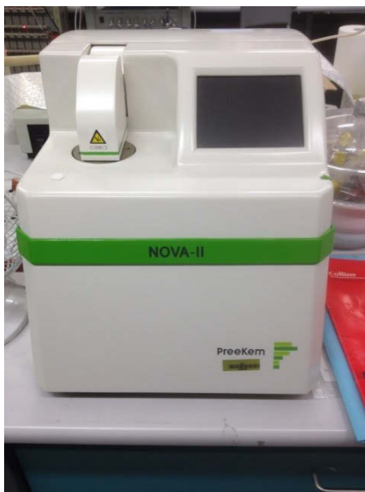
Figure 2- 5 Single-mode microwave synthesizer with pressure and temperature controllers
