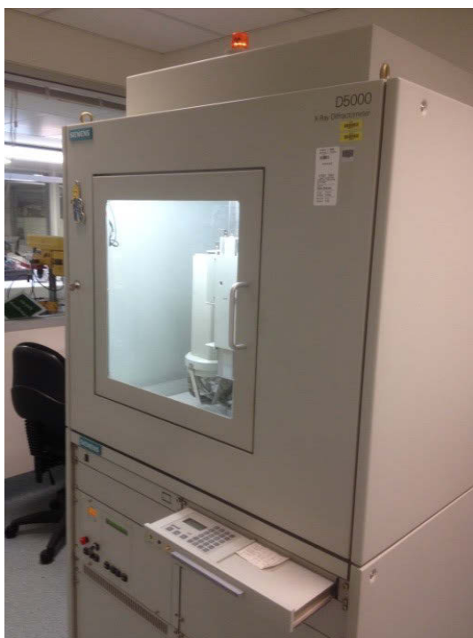
Figure 2- 7 Siemens D5000 diffractometer for XRD measurements.
