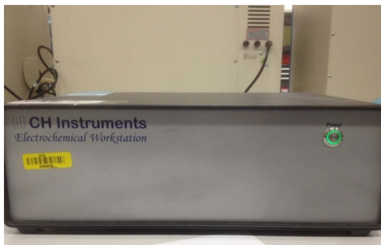
Figure 2-15 The CH instruments (CHI 660D) for CV and EIS testing.
