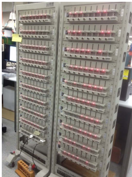
Figure 2- 14 The computer-controlled Neware battery test system.
