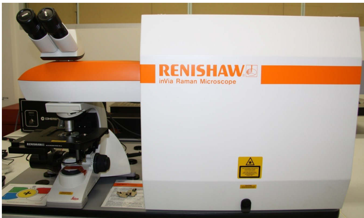
Figure 2-9 The Renishaw inVia Raman microscope equipped with a Leica DMLB microscope (Wetzlar, Germany) and a 17 mW at 633 nm Renishaw helium neon laser.
