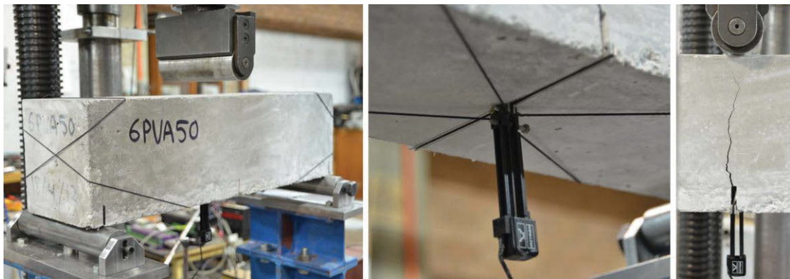
Figure 69. Residual flexural tensile strength test
