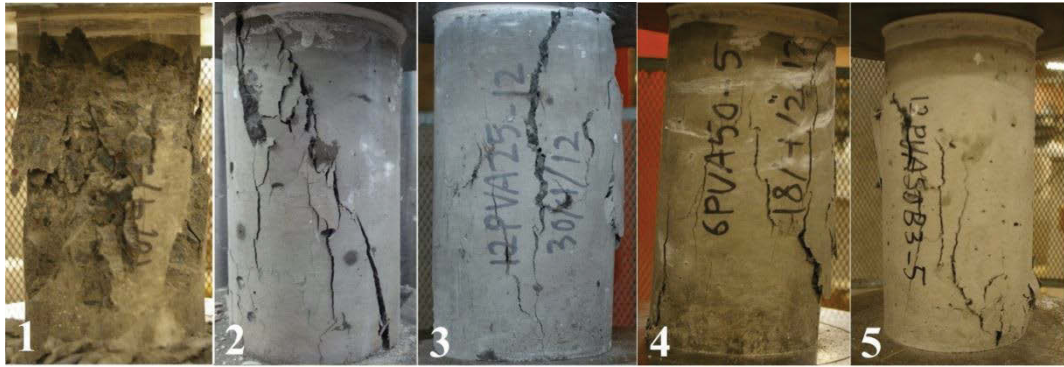
Figure 56. Compression failure modes of FRCs and control at 28 days
