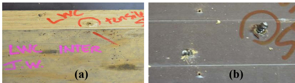
Figure B-33 (a) Failure of tensile screw (b) tensile failure of screw Scoria LWC SFS I45
