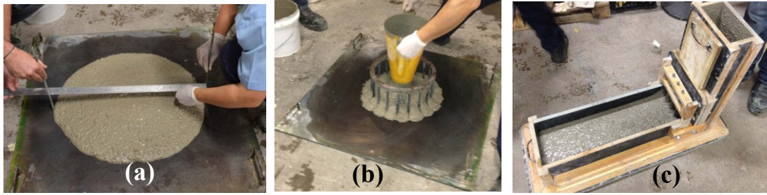
Figure A-1 (a) Slump-flow (b) J ring and (c) L box tests to measure workability of SCC
