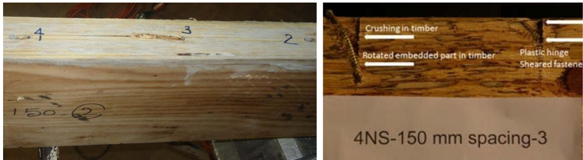
Figure 10-12 Opened specimens and failure mode of four wood screws at 150mm
