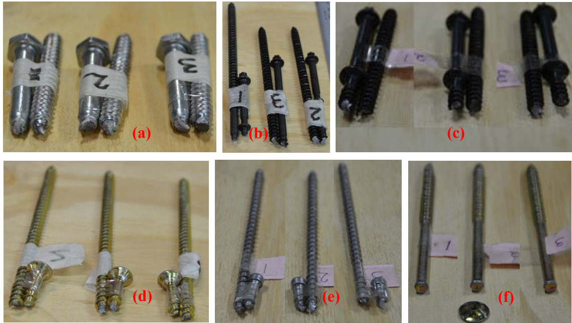
Figure D-2 Tensile failure of (a)medium coach, (b)long SFS, (c)short SFS, (d) SPAX, (e)small SPAX screws and(f)pull-off failure of type17 wood screw used in TCCs
