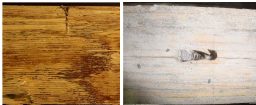
Figure 10-11 Opened specimens and failure mode of single wood screw
