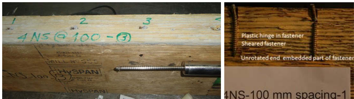
Figure 10-13 Opened specimens and failure mode of four wood screws at 100mm
