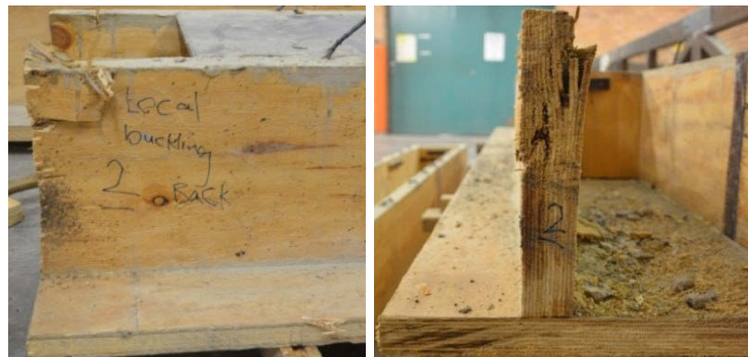
Figure 6-15 Local buckling of web underneath load cell at timber module 2
