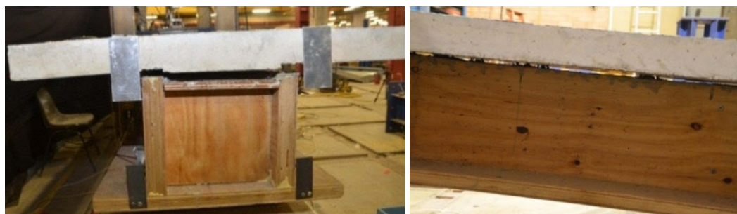
Figure 6-23 Uplift of the concrete slab relative to the timber joist
