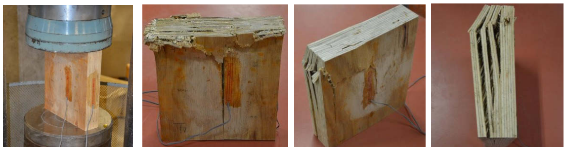
Figure A-16 Test set-up and compressive failure of LVL loaded parallel to the grain
