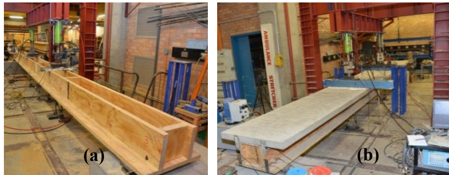
Figure 6-5 The layout of specimens: (a) the timber-only and (b) TCC modules
