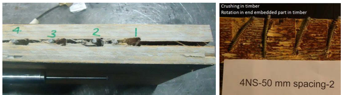
Figure 10-14 Opened specimens and failure mode of four wood screws at 50mm
