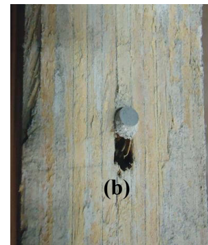
Figure 9-16 (a) FEM displacement in y direction and (b) failure of single wood screw
