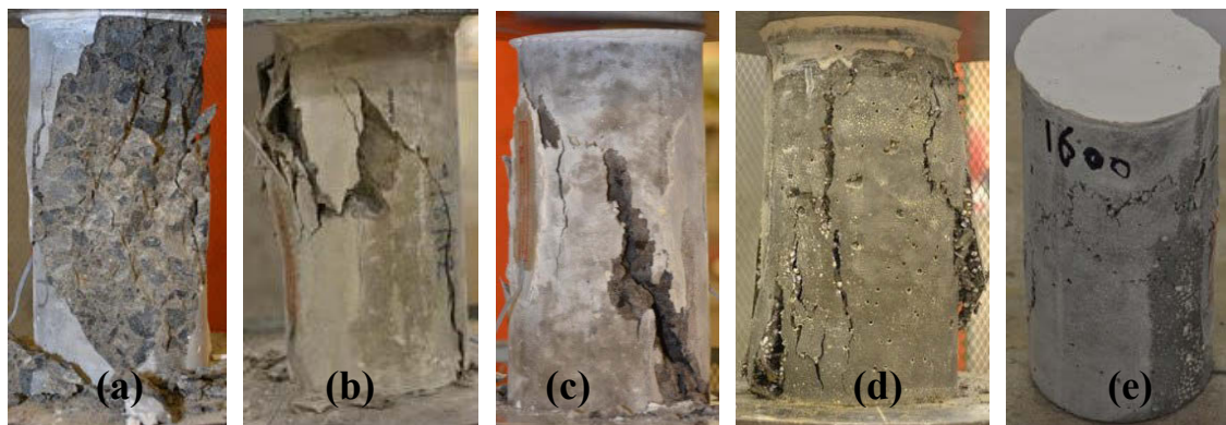
Figure A-7 Failure mode of (a) HSC, (b) CC, (c) Scoria LWC, (d)EPS LWC2000 and (e) EPS LWC1600 in compression
