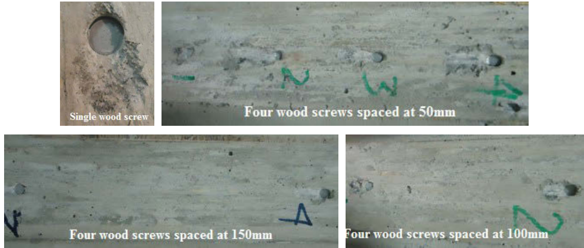
Figure 10-15 Concrete crushing in different series
