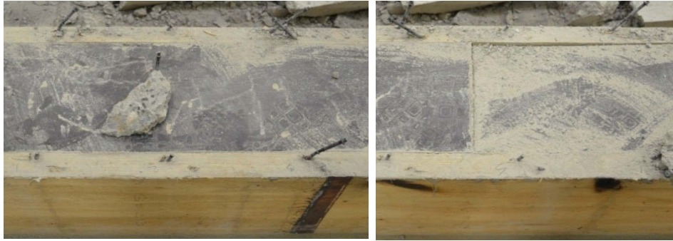
Figure 6-21 Failure of the first six pairs of SFS screws
