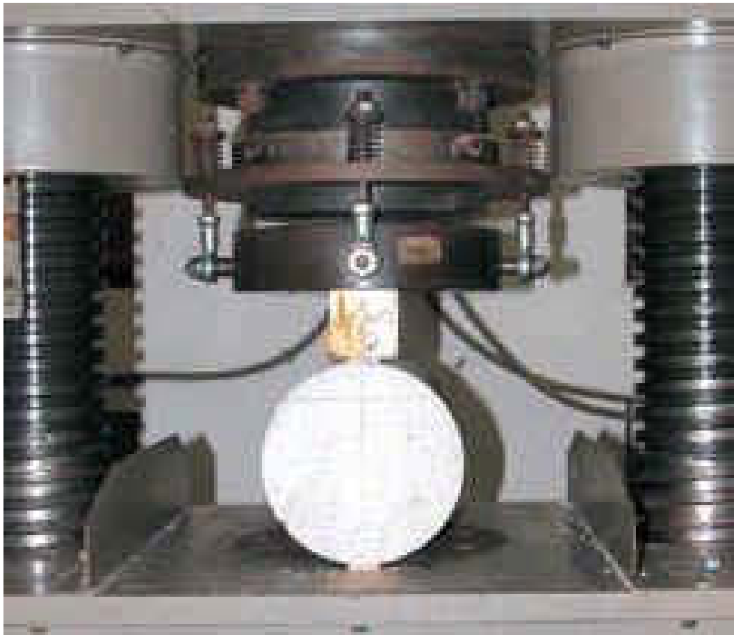
Fig. 3.8: Set up of splitting tensile test using a hydraulic pressure machine
