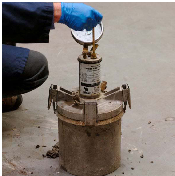
Fig. 3.6: Measuring air content of fresh concrete
