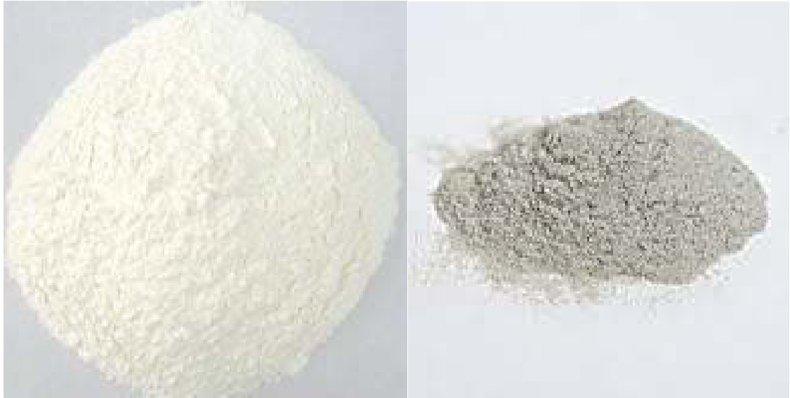
Fig. 3.1 : Sample of silica fume (left) and pumice (right)
