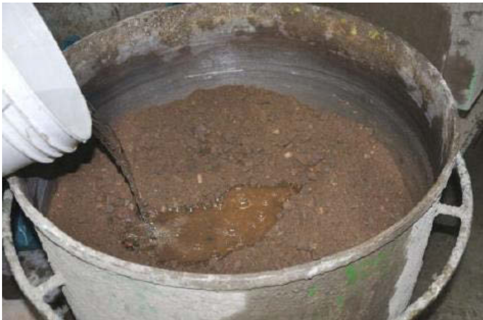
Fig. 3.3 : The time of adding water to mixture in a rotating pan mixer
