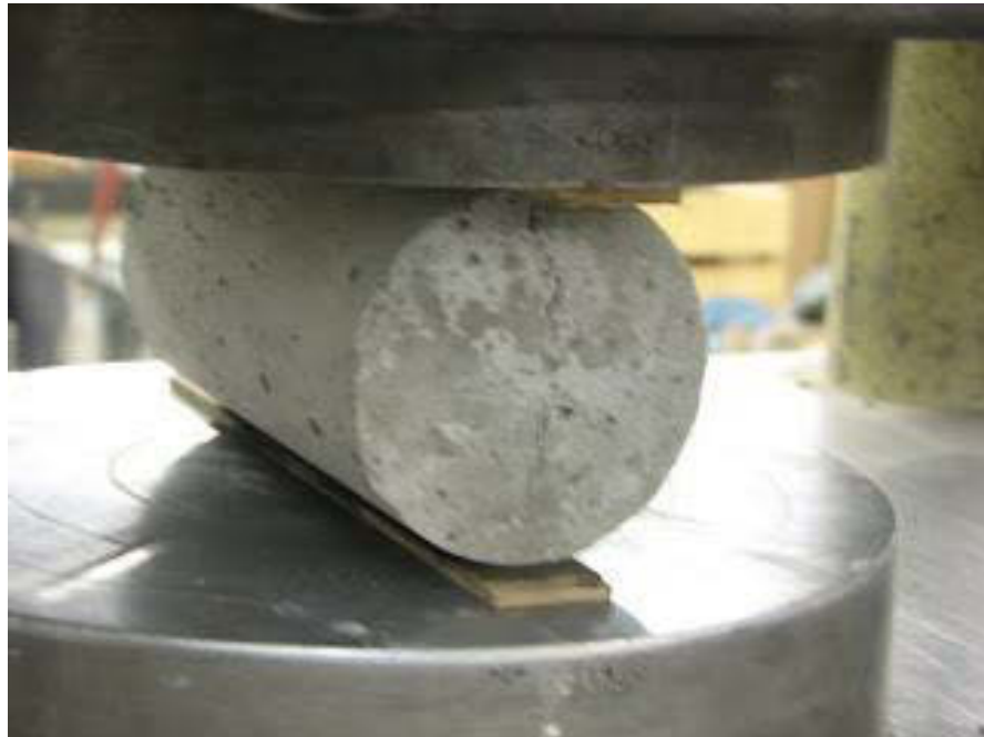
Fig. 3.9 : Specimen is located between two plywood strips for splitting tensile test
