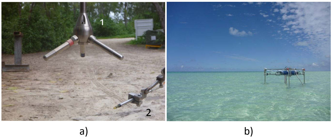
Figure 1.3: a) EC system components: ADV (a1) and oxygen optode (a2); b) EC system deployed on Heron Island.
