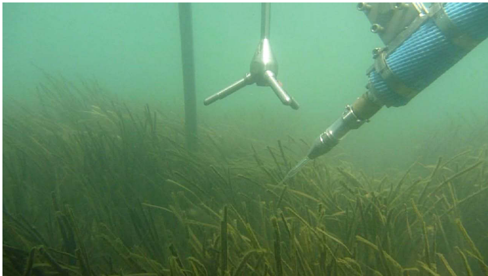
Figure 4.3: The deployment of the first generation of the Eddy Correlation microelectrode system (ECE1) in Tweed River seagrass beds.
