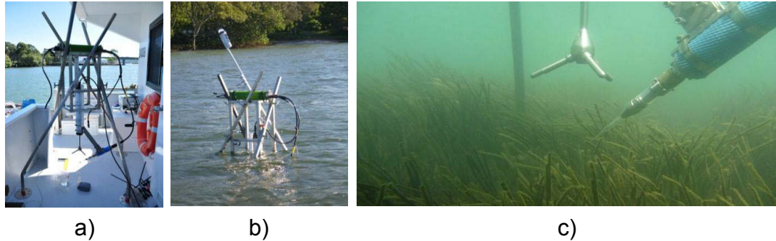
Figure 2.19: a) The EC mounted on the first version of the EC frame; b) The EC deployed in the Tweed River; c) The EC above the seagrass canopies.
