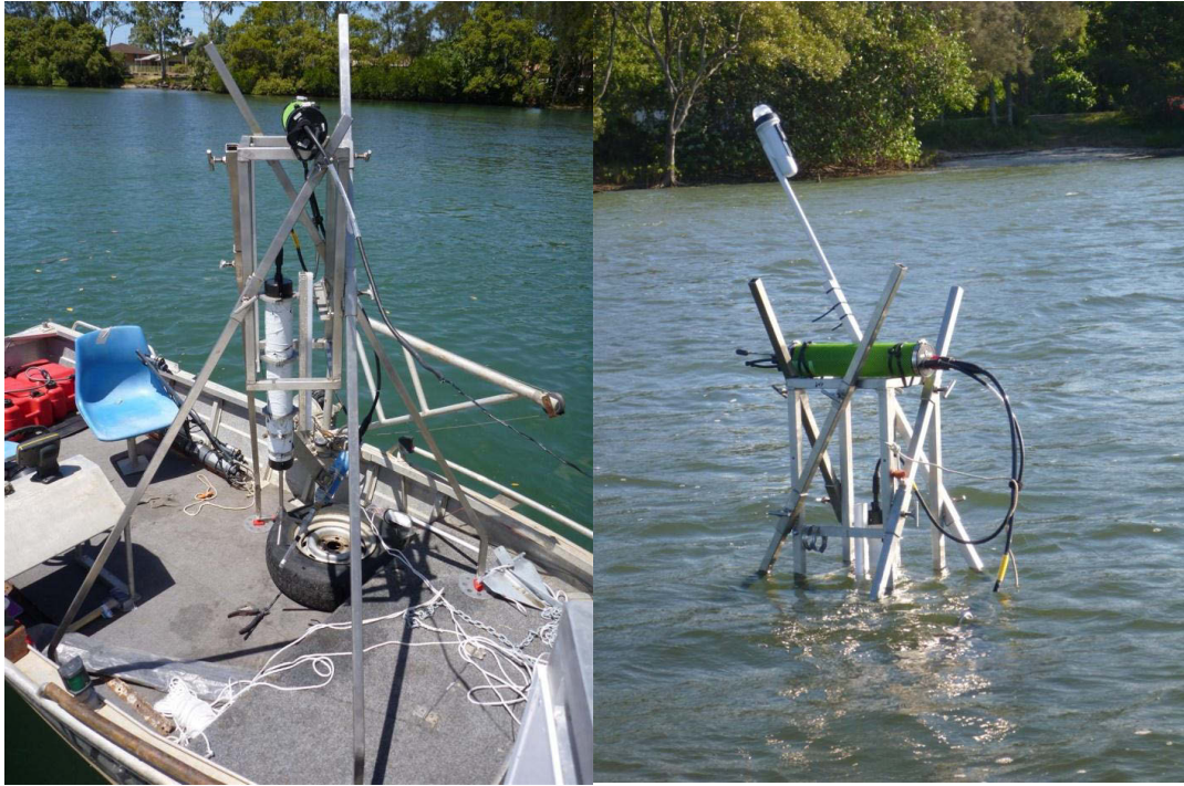
Figure 4.2: The first generation of the Eddy Correlation microelectrode system (ECE1; left) and the ECE1 during deployment in the Tweed River (right).
