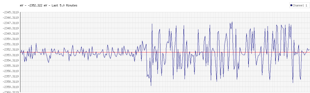
Figure 2.3: Two examples of electrical noise randomly appearing in the O 2 raw signal measured by ECE during laboratory experiments.
