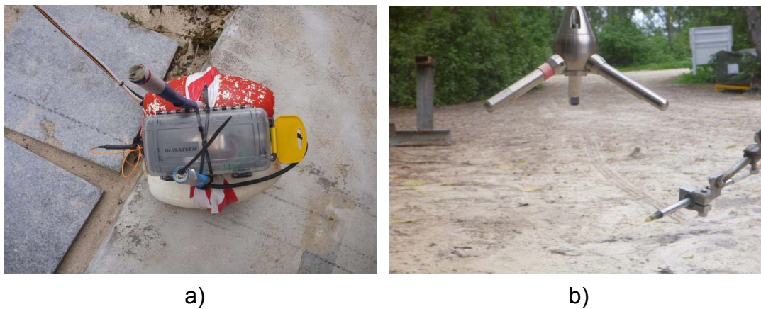
Figure 2.5: a) A custom-made splash-proof housing for FireSting; b) A fast optode.
