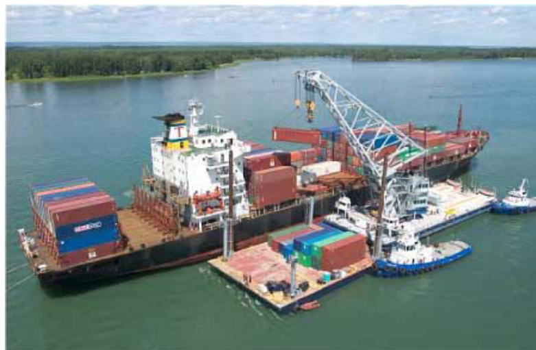
Figure 1.3 : An offshore crane transferring containers between a ship and a vessel [135].
