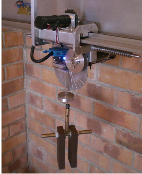
Figure 4.1 : Two-dimensional gantry crane system at UTS laboratory.
