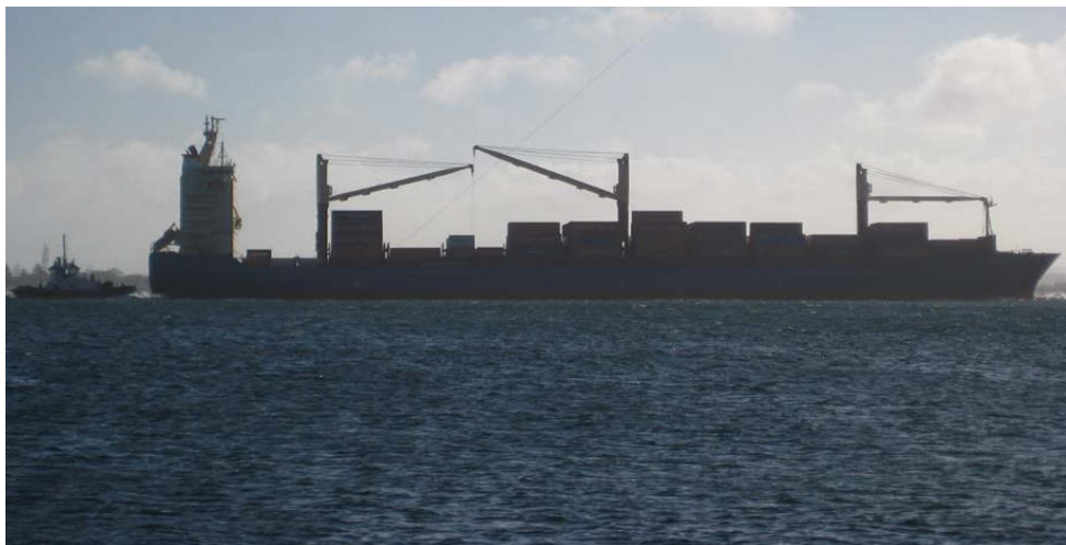
Figure 1.5 : Ship-mounted boom cranes near Port Botany, Sydney.
