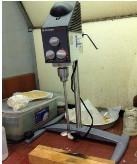
Figure 3–1 Bench–scale agitator used for conditioning tests in the study
