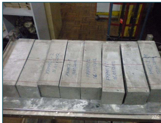
Figure 7-8 Specimens after flexural test
