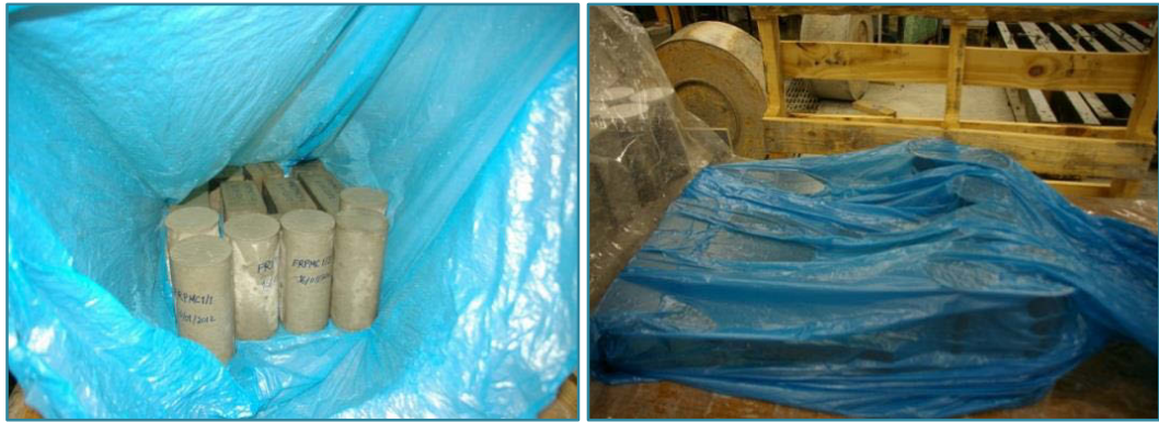
Figure 6-18 Moisture curing of PMC and FRPMC specimens for 48 hours
