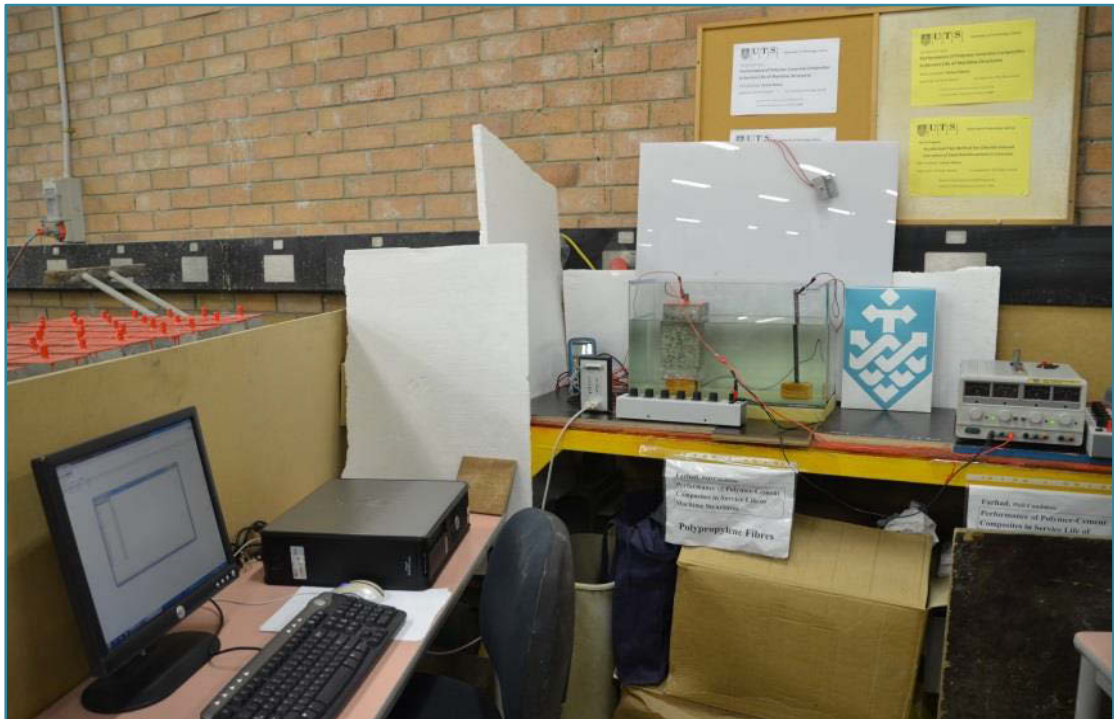
Figure 6-35 Time to corrosion-induced crack laboratory test set up
