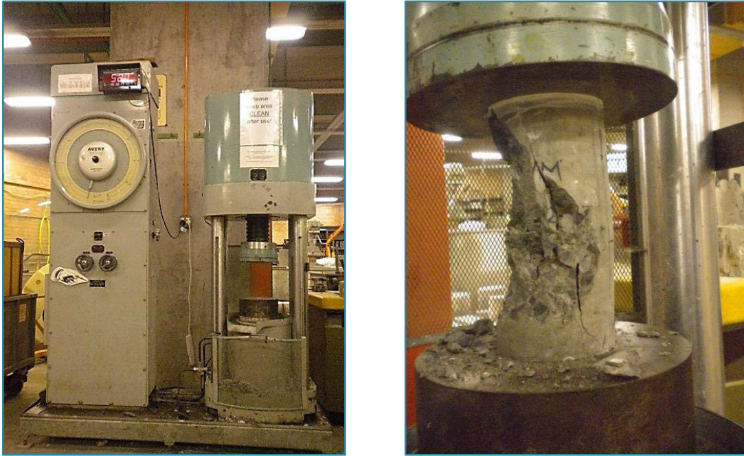
Figure 6-24 Compressive test machine
