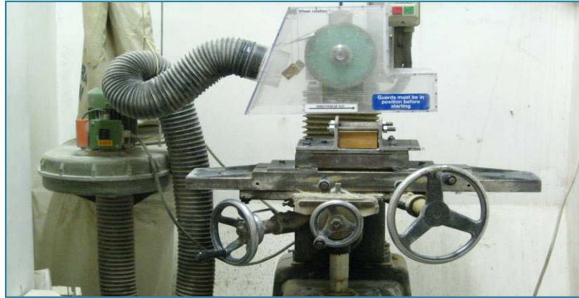
Figure 6-29 Concrete grinding machine
