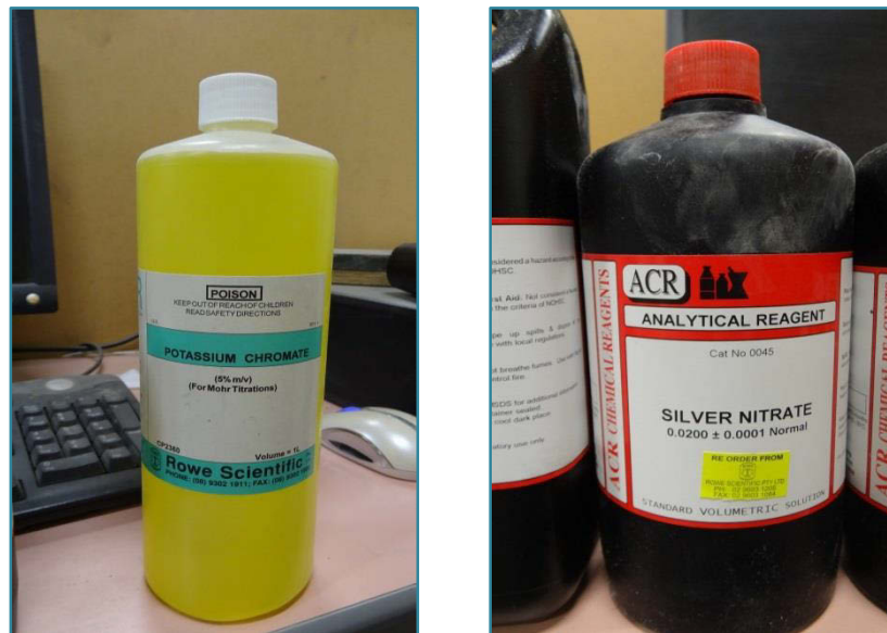
Figure 6-31 Potassium chromate and silver nitrate solutions for identifying concentration of chloride ions in salt solution
