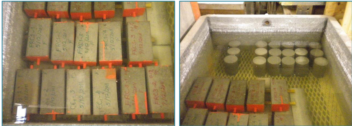
Figure 6-17 Curing method for CC and FRC specimens
