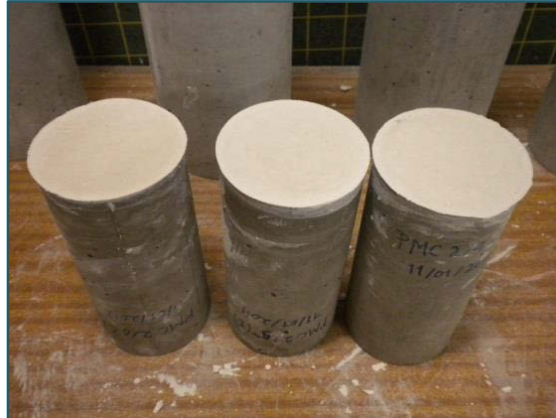
Figure 7-2 Capped specimens by gypsum for compressive strength test
