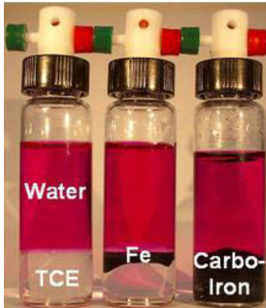
Figure 2-6: Picture showing the high affinity of nZVI for hydrophobic compounds (i.e. TCE) when combined with activated carbon (Kopinke and Mackenzie 2012).
