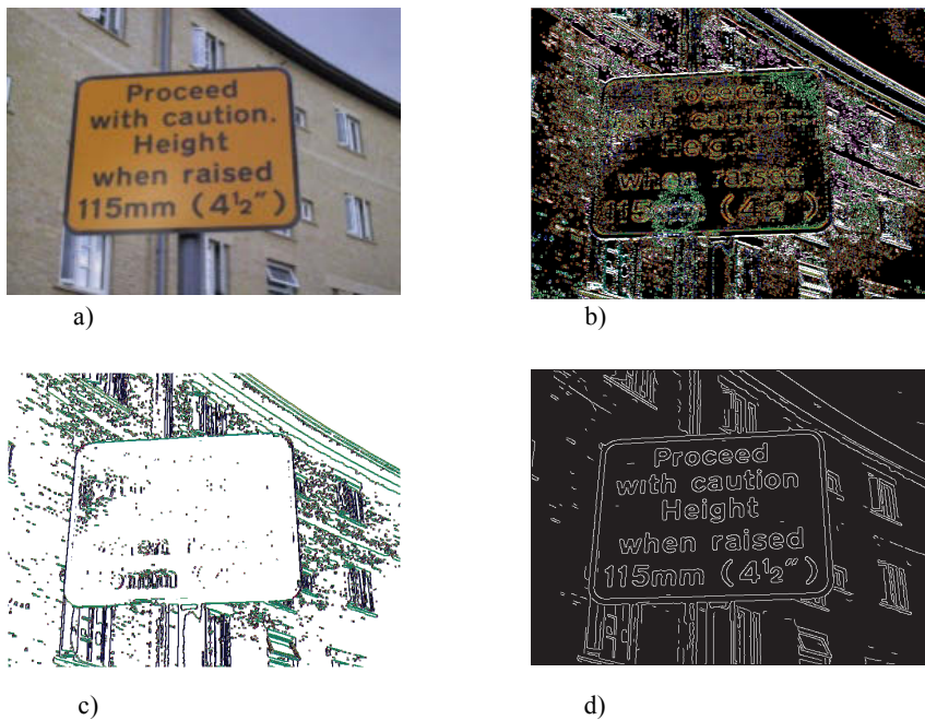
Figure 2.7 a) Original image. b) Traditional (Sobel) edge map. c) Kirsch edge detector; d) Edge map with embedded confidence
