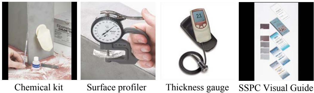
FIGURE 2.3: Commercial surface inspection instruments [3], please refer to Appendix D for SSPC visual guide
