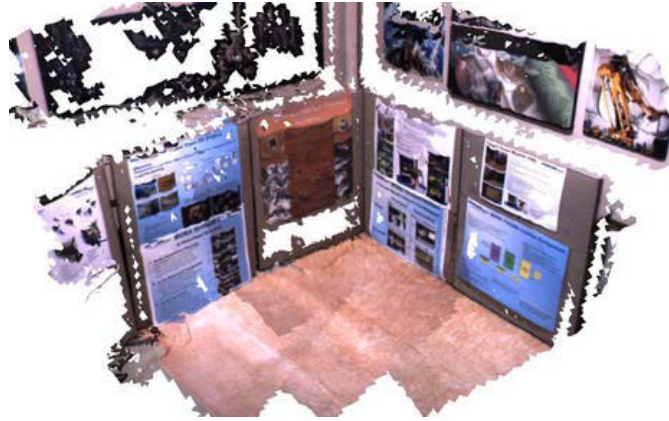
FIGURE 2.1: 3D geometric map with additional colour information [1]
