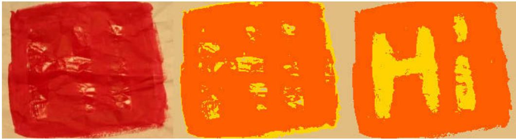
FIGURE 2.8: Captured sample image (left), Classification based on single image (middle), Classification based on Hemispherical Harmonic coefficients (right) [12]
