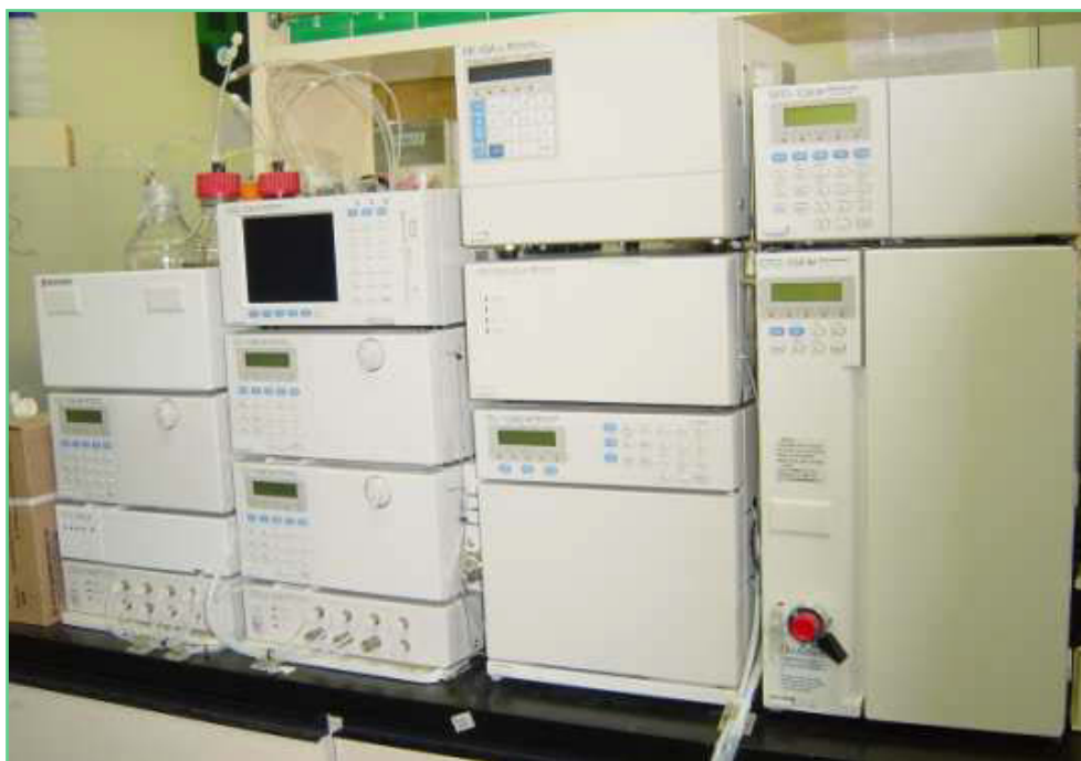
Figure 3.10 High pressure size exclusion chromatography (HPSEC) to measure MW distribution
