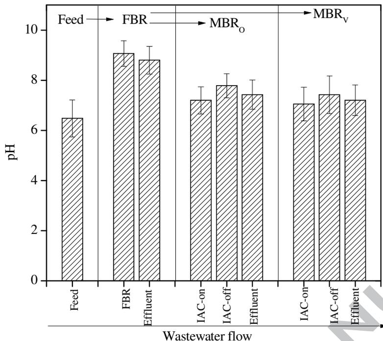
**Fig. 1.** The pH values ( $n=72$ ) of feed, FBR, MBR and effluent that operate at optimum ( $MBR_O$ ) and variable ( $MBR_V$ ) conditions. IAC-on and IAC-off is used to indicate pH measurements carried out in the MBR under air pump working and pausing periods, respectively. The MBR effluent pH was the combined result that flows during “on” and “off” cycles.
