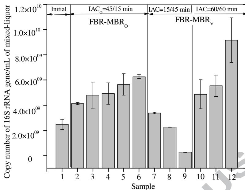
**Fig. 4.** Total bacterial copy numbers of 16S rRNA gene per mL of mixed-liquor for initial (sample 1), 45/15 min (sample 2, 3, 4, 5 and 6 collected at day 30, 60, 90, 120 and 150, respectively), 15/45 min (sample 7, 8 and 9 collected at day 30, 60 and 90) and 60/60 min (sample 10, 11 and 12 collected at day 30, 60 and 90) aeration cycles for FBR-MBR combo systems as revealed by the SYBR Green I based qPCR method.
