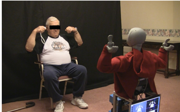
Figure 3.6: Assistive robot to deliver arm exercises for the elderly (Fasola and Mataric, 2010)
