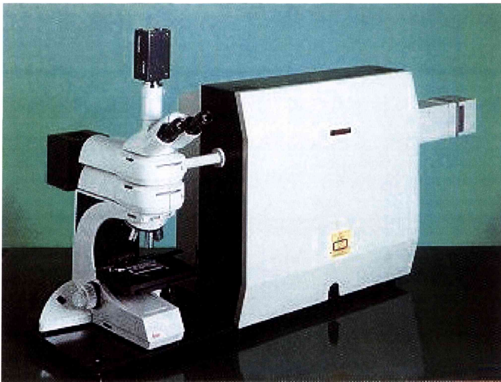
Figure 2-5 The 'Renishaw' Raman Spectroscopy System 2000, external view [130]
