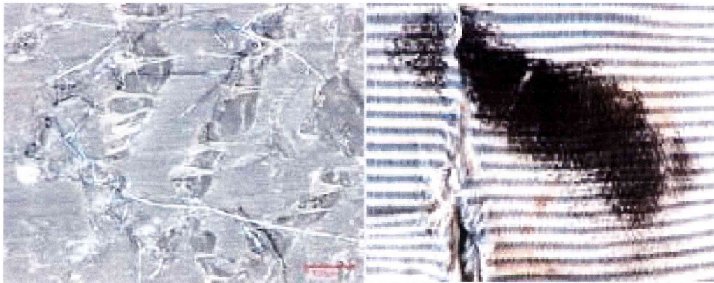
Figure 1-11 Examples of (left) Fibre Plastic Fusion, and (right) Plastic Coating Mark (reprinted from [34])
