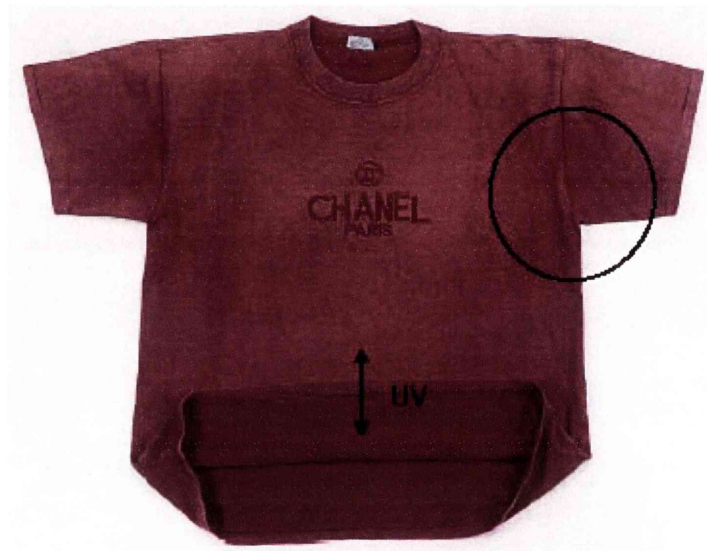
Figure 1-10 T-Shirt showing variations due to normal wear and tear (UV light damage indicated by areas circled) [33]
