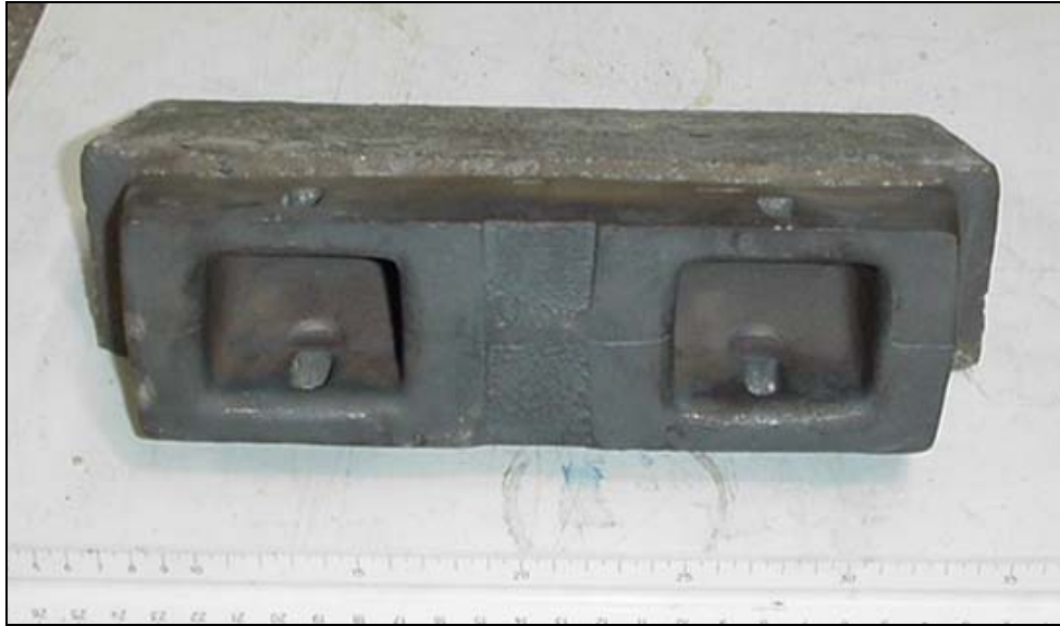
Figure 5.41: End view of wide bucket lip showing excellent bonding around the complete part
