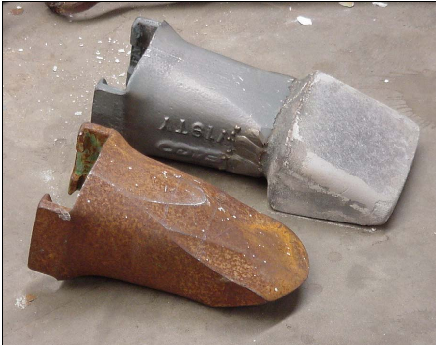
Figure 5.27: Original as-received steel part and new wide tip composite wear part
