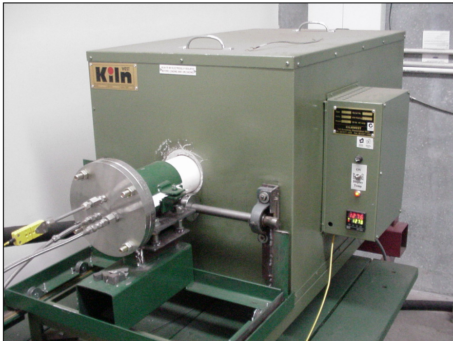
Figure 3.16: Vacuum tube furnace used for experimental development of the vacuum casting process
