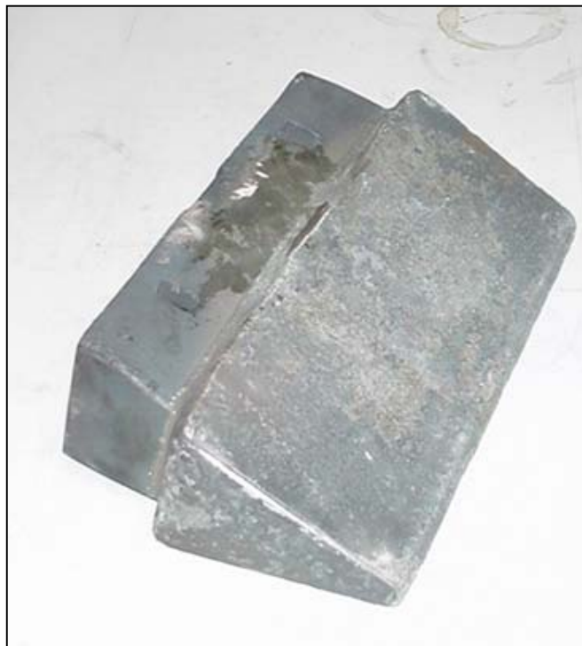
Figure 5.40: View of the finished composite wide bucket tooth prior to final painting
