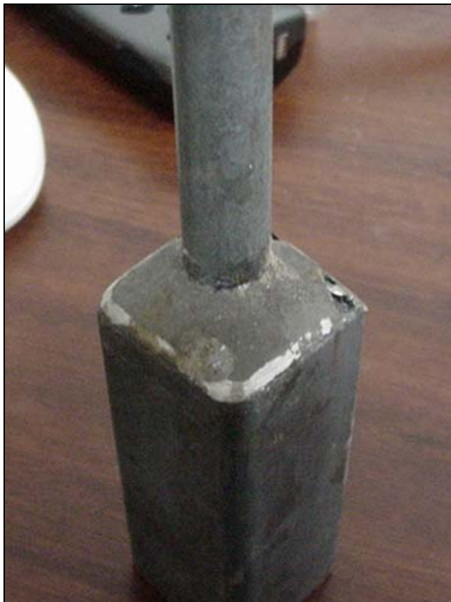
Figure 5.53: Detail of bonding/interface between centre rod, white cast iron and outer shell of composite tensile test sample
