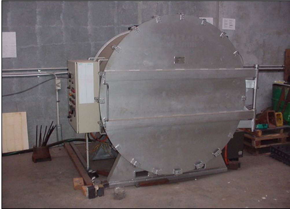
Figure 3.19: Hot wall vacuum furnace
