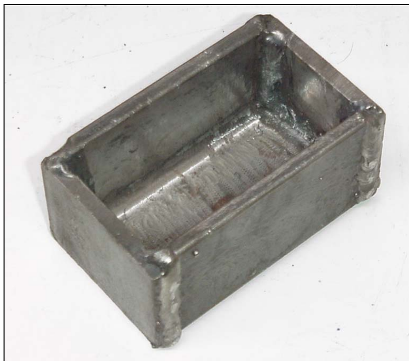
Figure 3.25: Prepared steel substrate after surface preparation and cleaning
