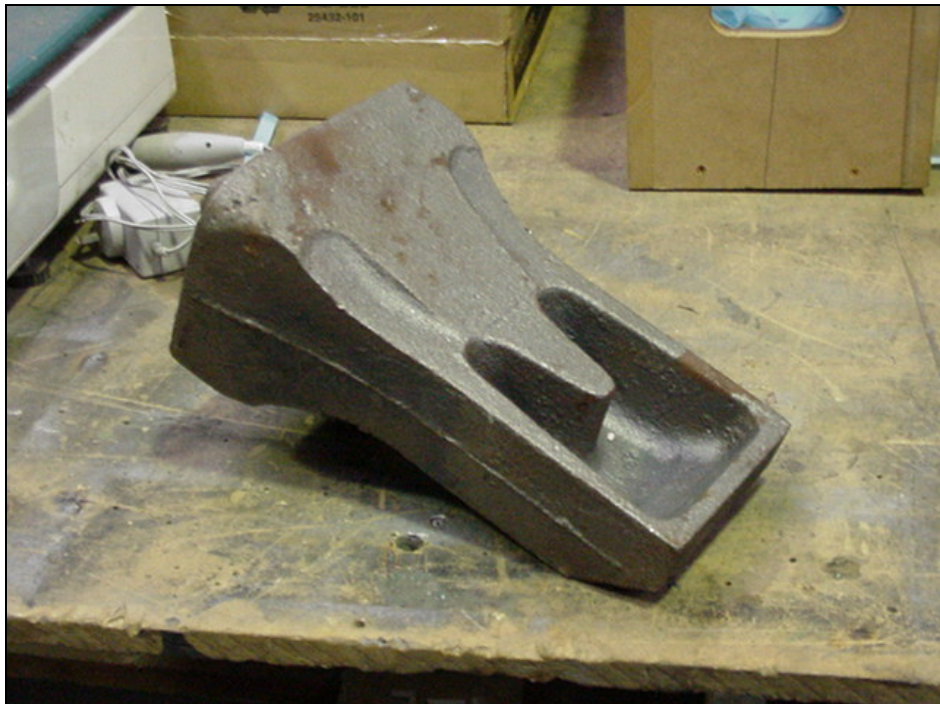
Figure 5.44: Cast chromium/molybdenum steel bucket tooth tip with cavity to receive white iron
