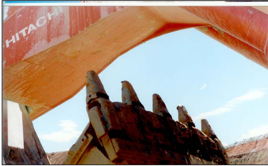
Figure 5.2: Typical bucket tooth installation on large mining excavator bucket
