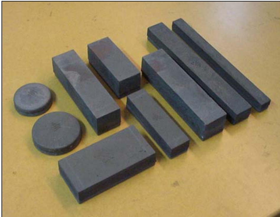
Figure 3.7: 75mm and 90mm buttons, 50mm x 50mm blocks of different lengths, 25mm x 25mm x 300mm bars, and other assorted sized blocks
