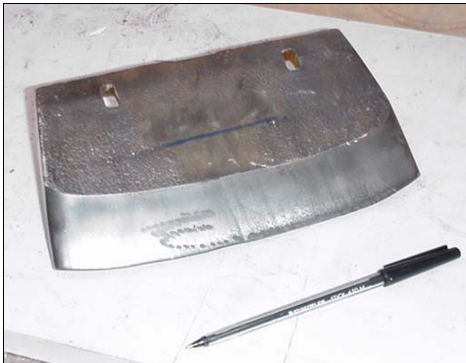
Figure 5.30: Worn steel dredge wide bucket lip
