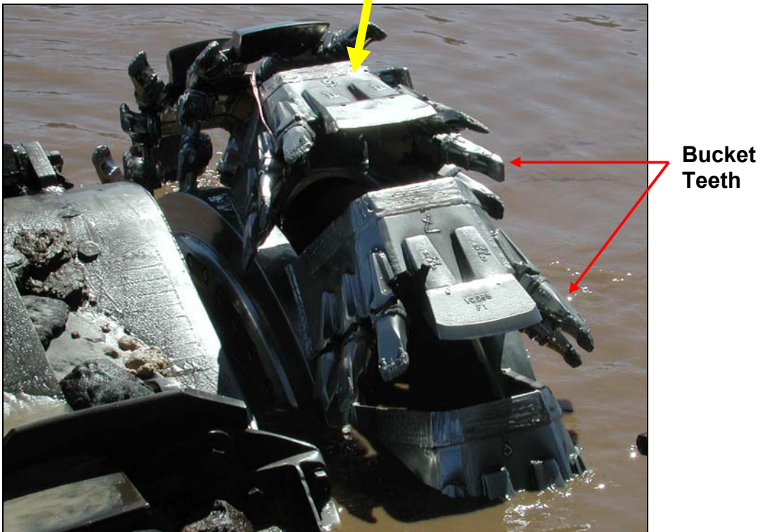
Figure 3.28: Typical suction-cutter dredge head (shown in the raised position)
