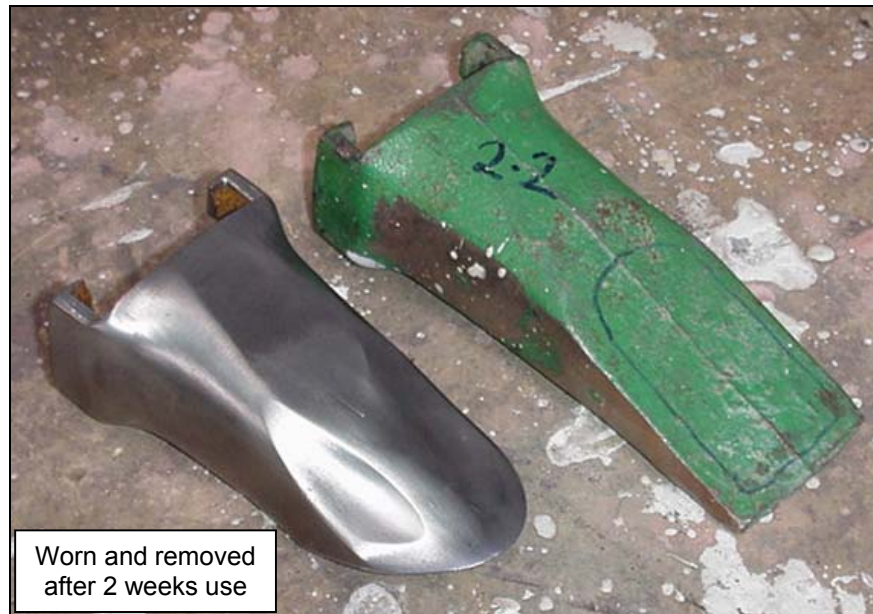
Figure 5.14: New and worn original Cr/Mo steel dredge bucket teeth (ESCO V19TY)
