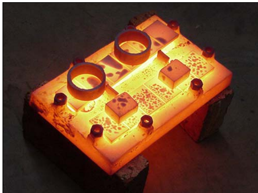
Figure 5.46: Hot “chok” bar mould with cast parts after removal at 1000°C from furnace
