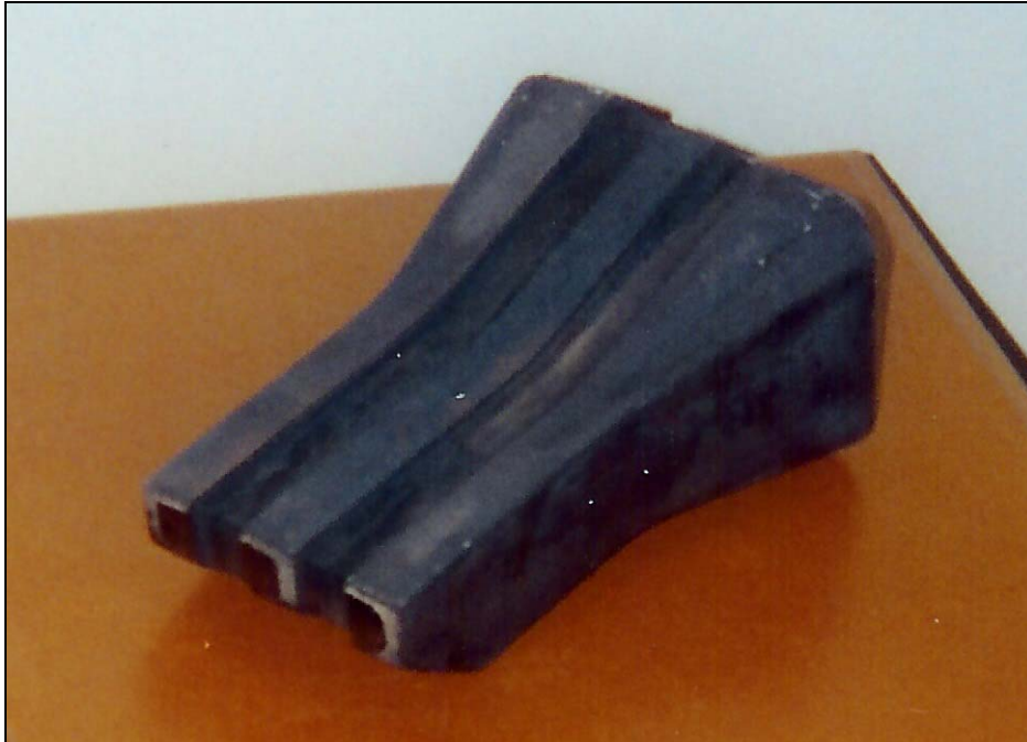
Figure 5.13: Finished vacuum brazed multi-laminated bucket tooth tip.
