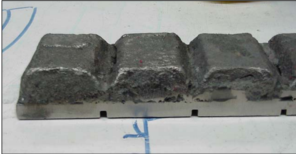
Figure 5.48: Detail view of excellent bonding between white cast iron and steel backing plate. Some minor edge gaps are present which need to be eliminated by future modifications to the method of moulding.
