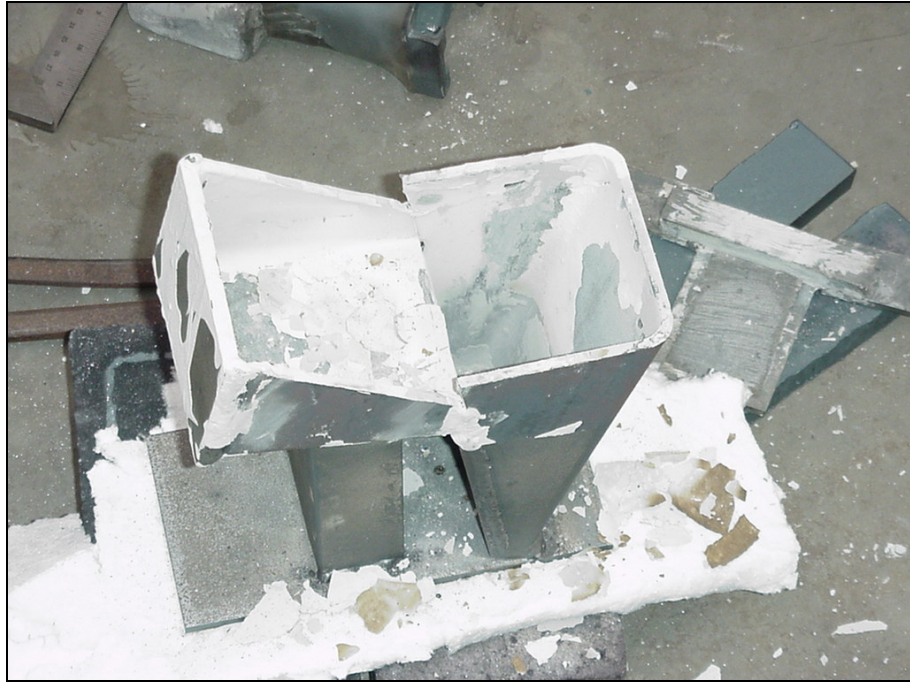
Figure 5.29: Ceramic coated mould after removal of the finished composite part
