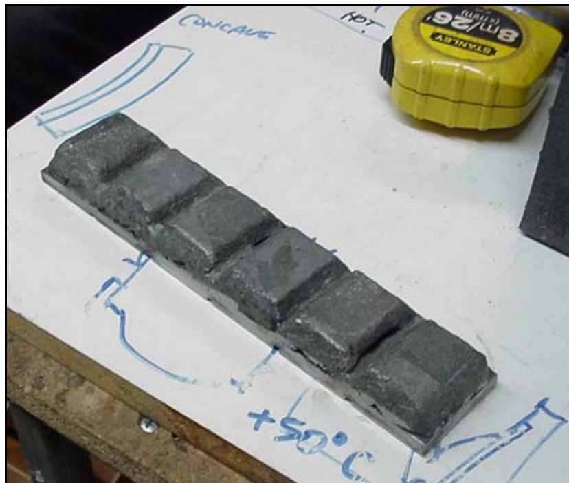
Figure 5.47: Finished composite white iron/steel “chok” bar after casting using vacuum based process
