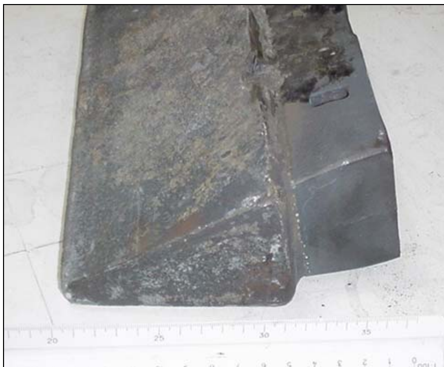
Figure 5.39: Finished composite wide bucket lip after removal from the mould
