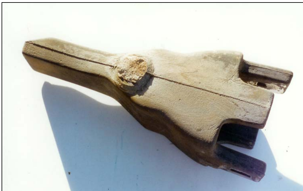
Figure 5.9: Full white iron cast bucket tooth (equivalent to ESCO V66RDX tooth)
