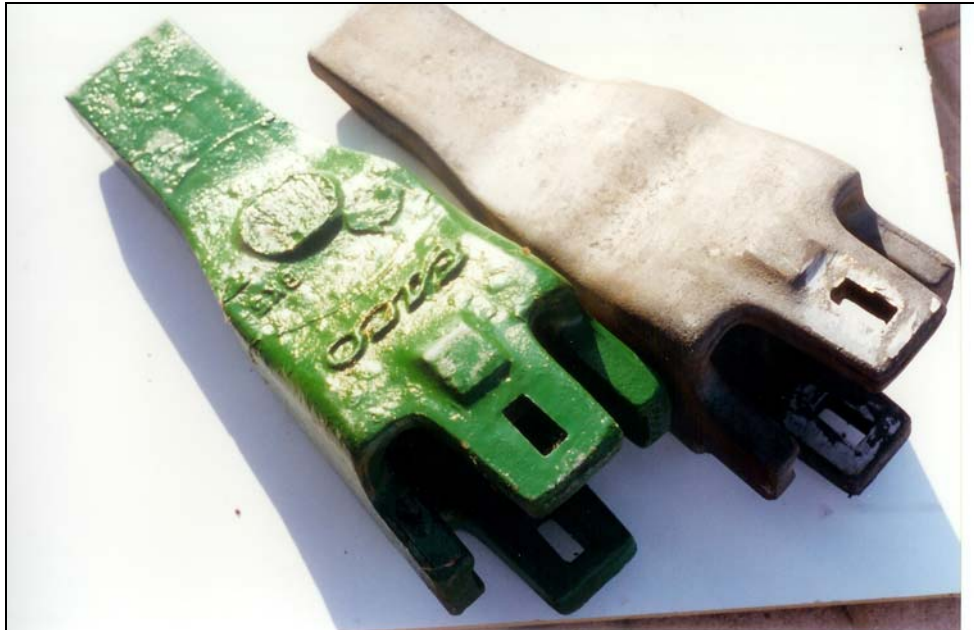
Figure 5.10: Comparison of cast white iron and cast steel bucket teeth
