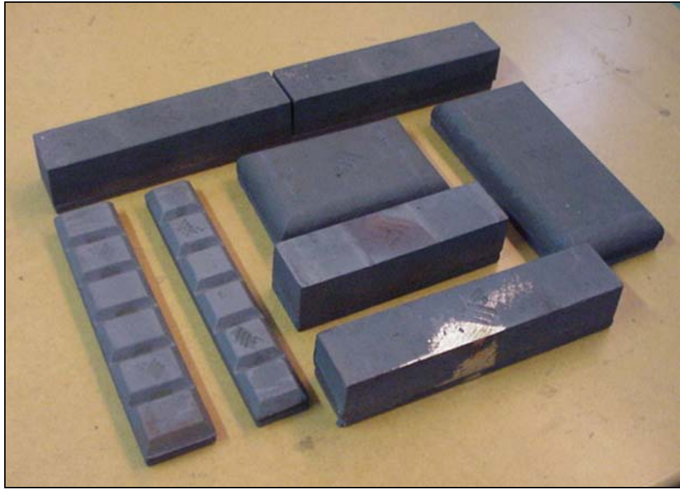
Figure 3.8: 50mm x 50mm x 432mm Block, 240mm x 50mm and 240x40 "Chok" Blocks, 50x50 blocks and two skid pads
