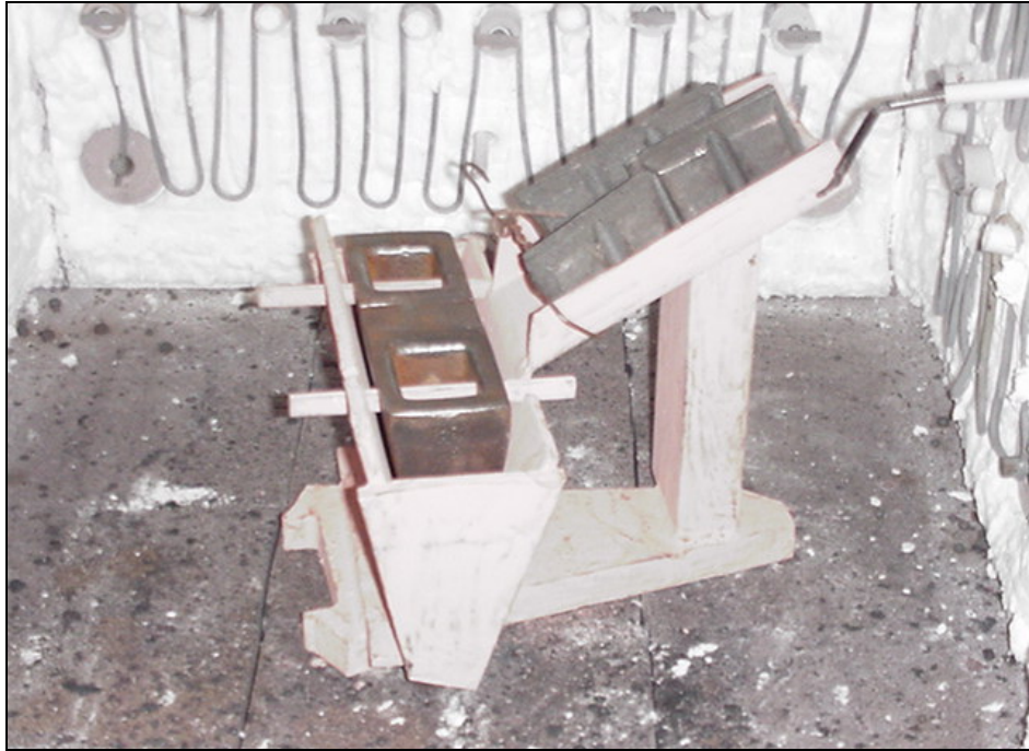
Figure 5.33: Wide bucket tooth lip part inserted into furnace ready to start the cycle
