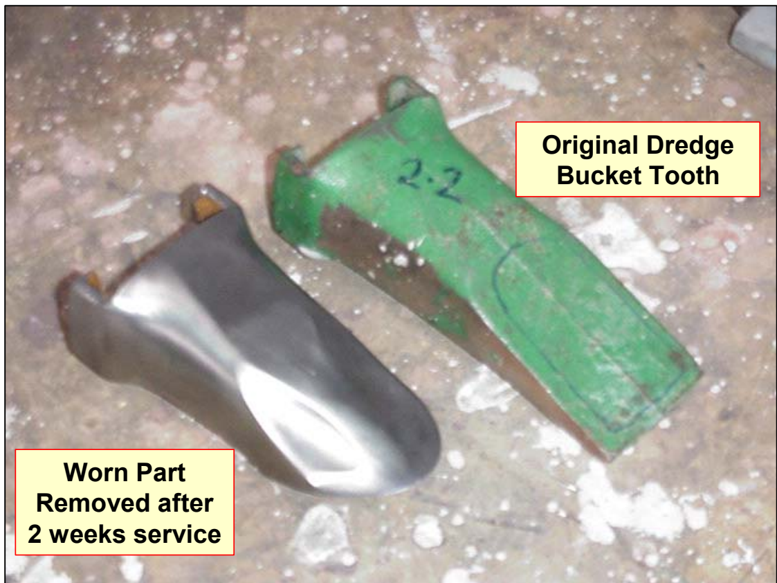
Figure 3.30: Typical original and worn steel bucket tooth used on the suction-cutter dredge.
