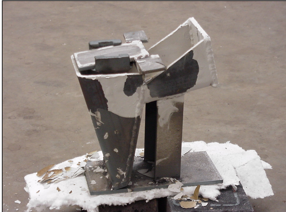
Figure 5.24: View of steel mould with steel part positioned using retaining plate. White iron charge is weighed and placed into chute on the right of the mould. During the heat treatment cycle, the white iron melts and flows down the chute and fills the mould cavity coming into contact with the steel part.
