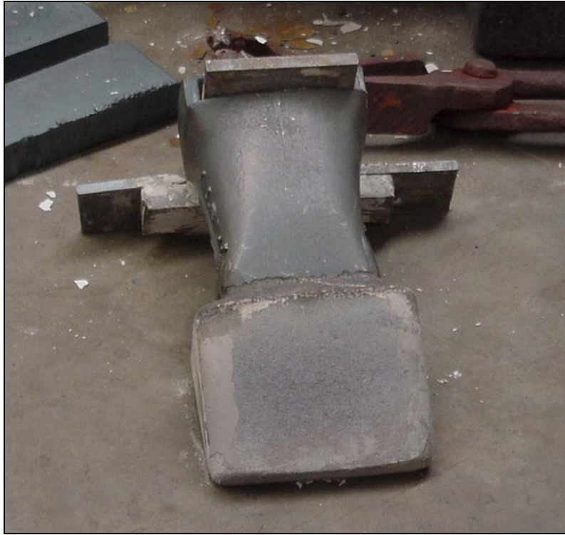
Figure 5.25: Completed wider tip composite part after removal from the metal mould
