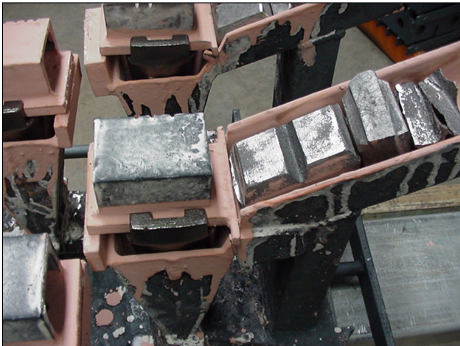
Figure 5.16: Closer view of steel part positioned with steel plate, and white iron charge located in side chute
