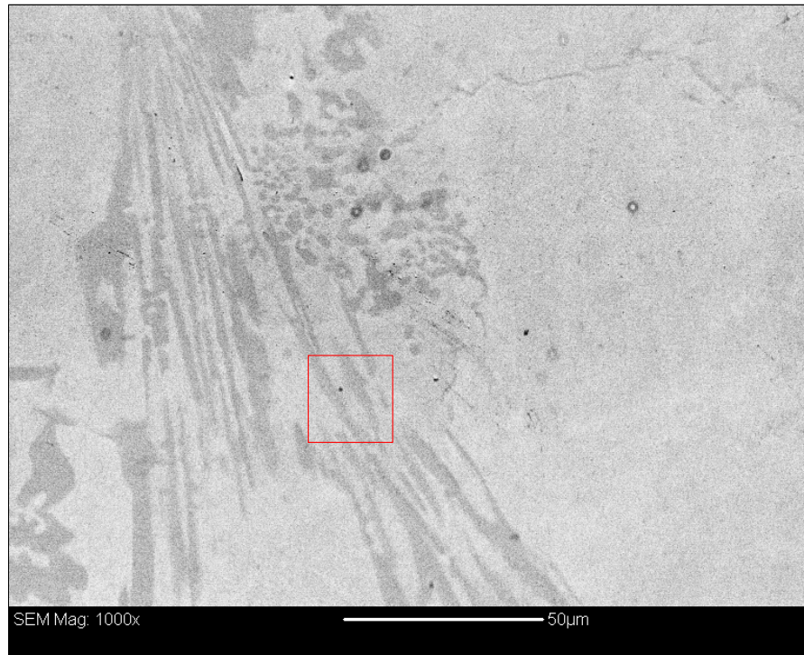
Figure 4.63: Location of higher resolution EBSD map for eutectic carbides in the white cast iron (Zone 4) of the vacuum cast composite.
