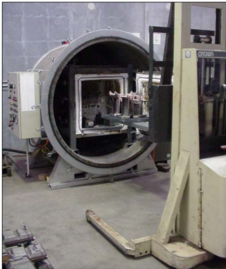
Figure 5.17: Loading the hot walled vacuum furnace with trial composite white iron/steel parts in steel moulds
