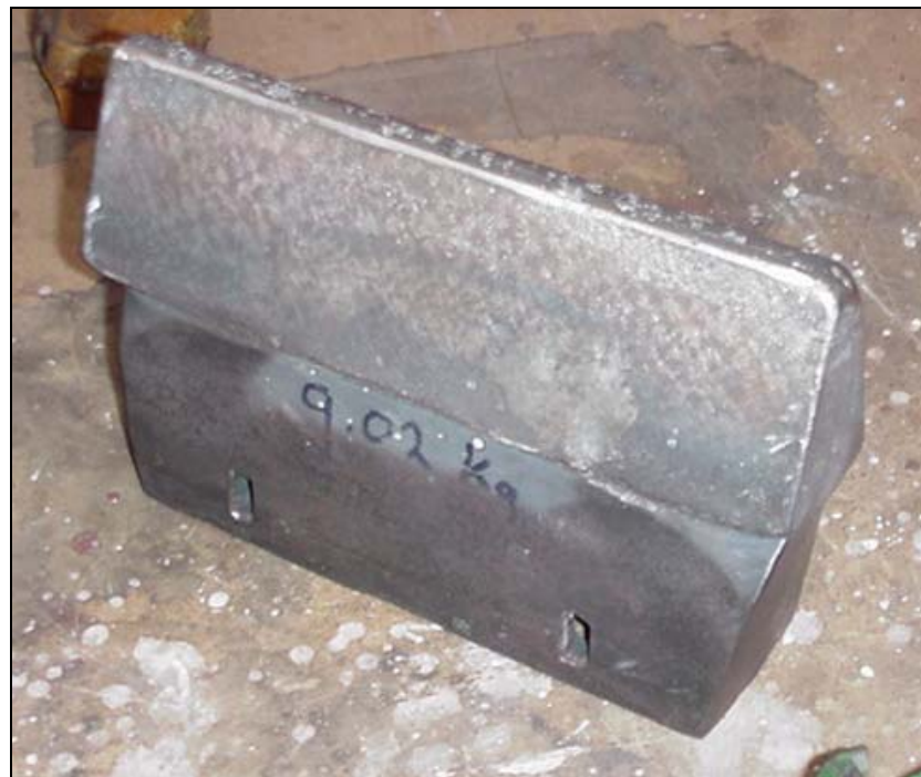
Figure 5.42: First production trial part with a final mass of 9.02kg. Subsequent cycles were adjusted for a total composite mass of 9.40kg.
