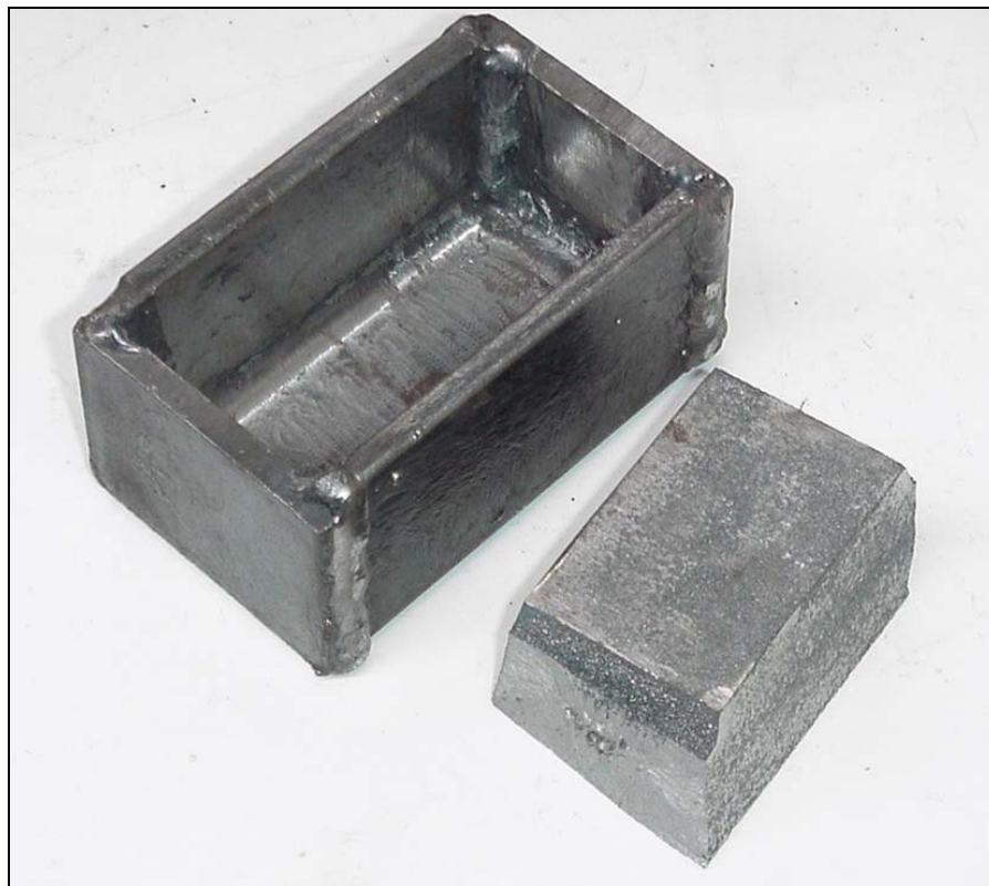
Figure 3.26: Prepared white iron Alloy C1 charge and steel substrate
