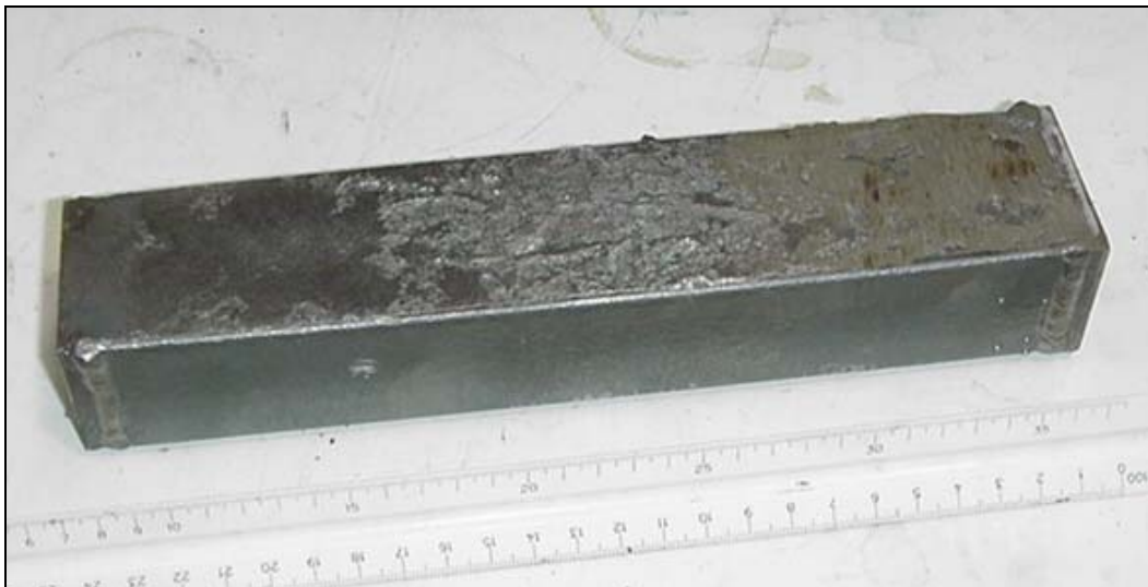
Figure 5.49: As-cast composite wear bar manufactured from "C" channel with welded end caps
