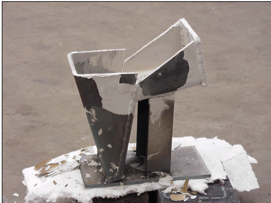
Figure 5.23: View of steel mould with ceramic coating on inside surfaces to assist with stopping bonding of white iron to the steel mould
