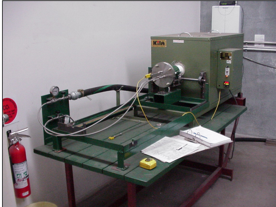
Figure 3.15: Vacuum tube furnace used for experimental development of the vacuum casting process
