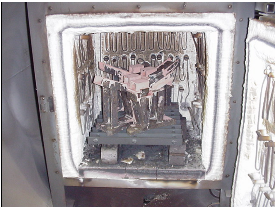
Figure 5.19: View of multiple steel moulds for composite white iron/steel parts placed into hot walled vacuum furnace
