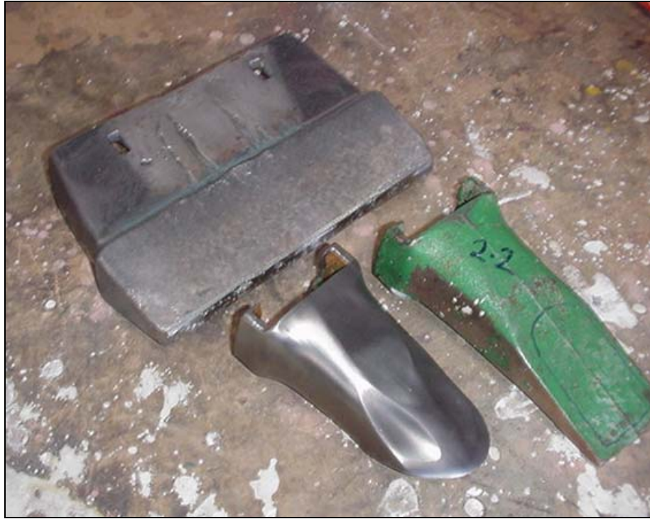
Figure 5.43: Comparison of sizes of wide bucket lip composite part to ESCO V19TY bucket teeth
