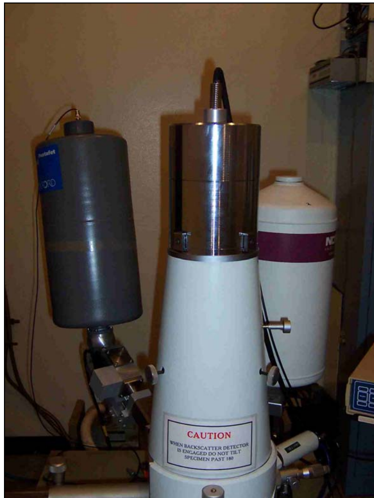
Figure 4.13: UTS Jeol 35CF fitted with two EDS detectors and Moran Scientific XRM System
