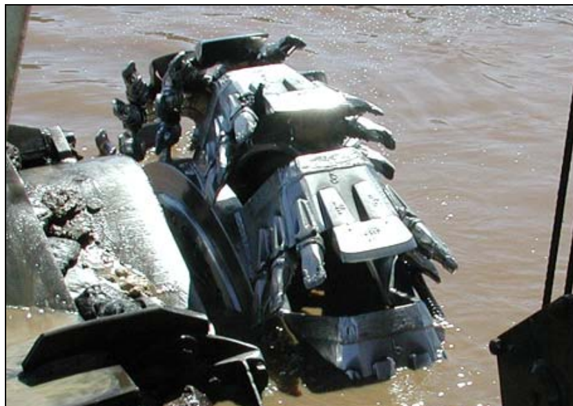
Figure 5.58: Closer view of bucket arrangement on suction-cutter dredge head. Note wide bucket lip and smaller side bucket teeth.
