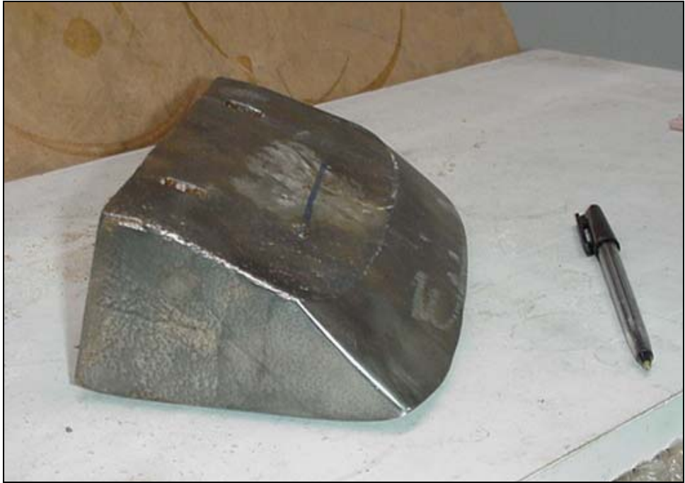
Figure 5.31: Side view of worn steel dredge wide bucket lip
