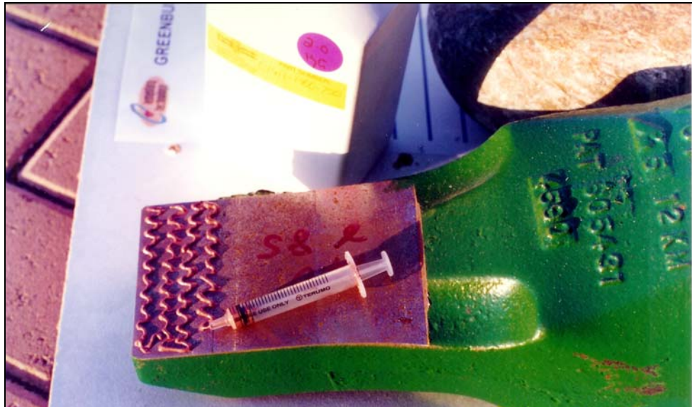
Figure 5.11: Machined V66RDX steel bucket tooth ready to vacuum braze white iron wear plate on front tip
