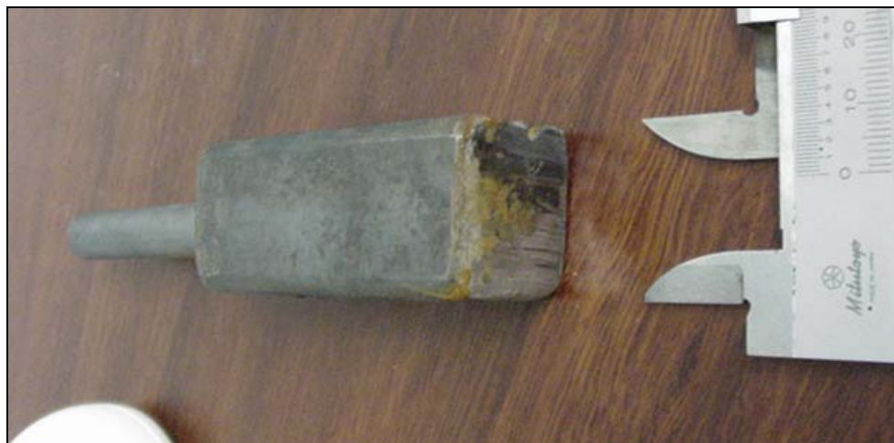
Figure 5.51: End view of completed composite debonding test sample
