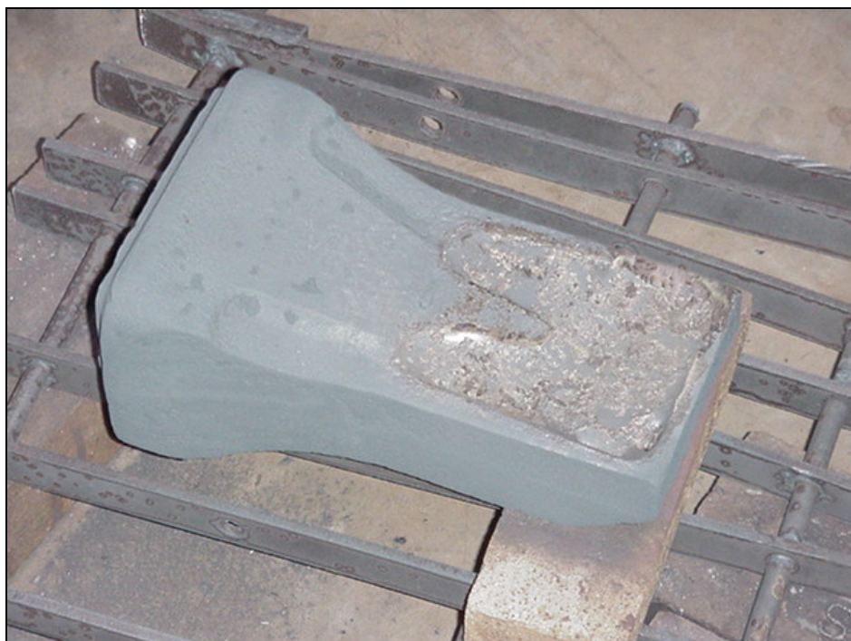
Figure 5.45: As-cast composite steel/white cast iron bucket tooth tip. Note the white iron has completely filled the cavity, and the absence of any significant surface scale.
