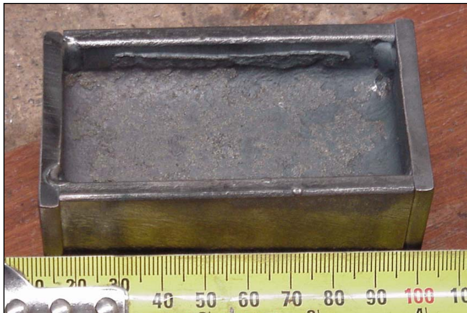
Figure 3.27: Typical bonded steel/white iron test sample after heat treatment in the vacuum tube furnace
