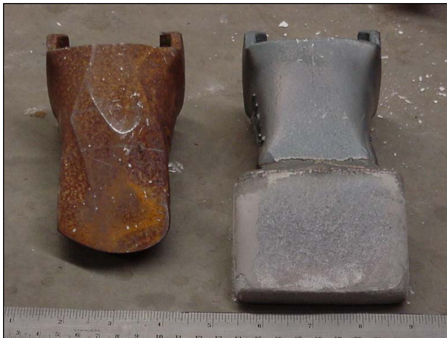
Figure 5.28: Front view of original as-received steel part and new wide tip composite wear part
