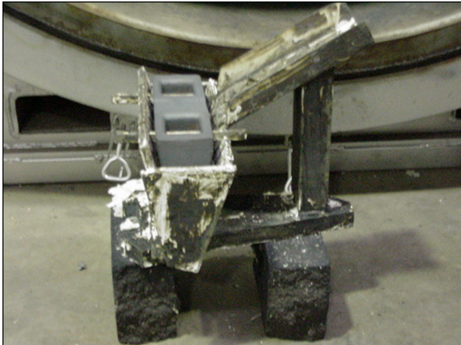
Figure 5.38: Side view of steel mould and composite part after removal from the furnace
