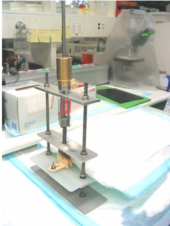
Figure 2.2 Image of closed fracture apparatus used in experiments.
