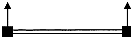
Figure 5–7: Boundary conditions of the crossbeams
