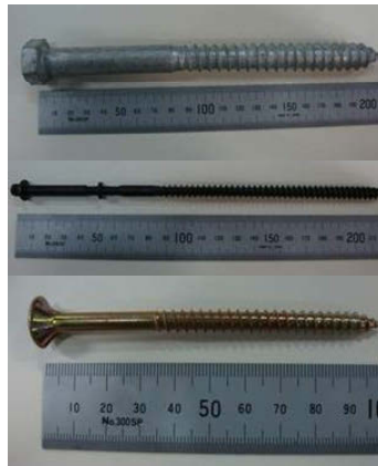
Figure 89 the lengths of the coach screw, SFS and normal screw used in the connectors
