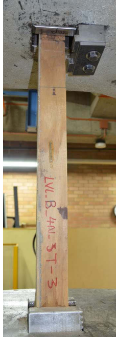
Figure 80: Set-up for tension test of LVL joist
