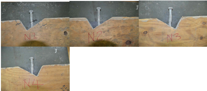
Figure 103 all the four connectors' investigation after failure for B-4N (N1 left end support, N2 left at L/4, N3 right at L/4 and N4 right support).
