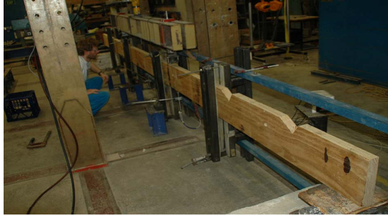
Figure 37: MOE test on LVL only
