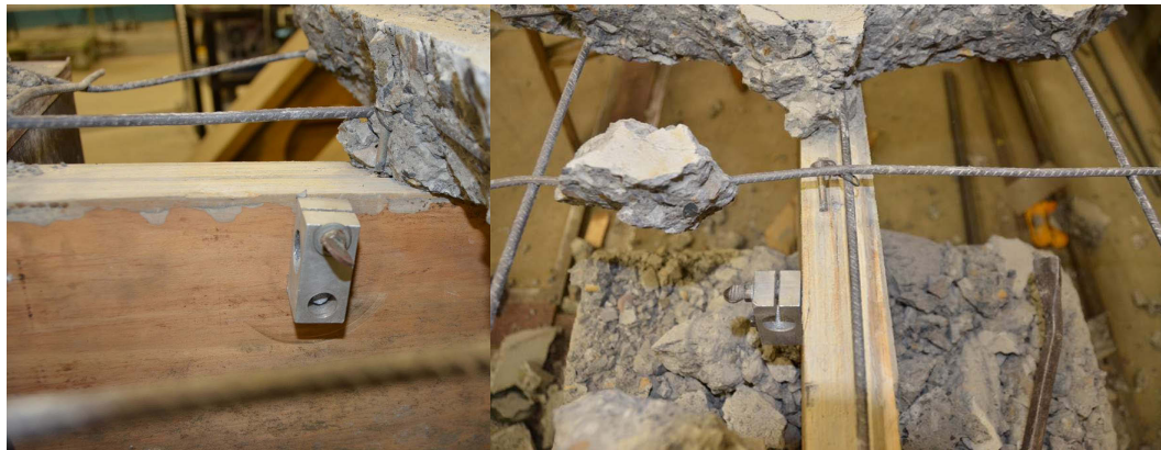
Figure 74 Connector close to the right support after failure for B-NS
