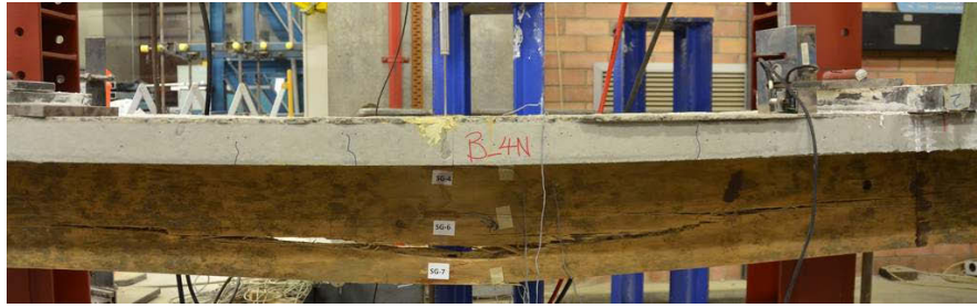
Figure 102 Failure patterns on the LVL for B-4N
