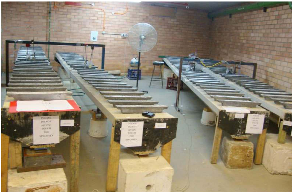
Figure 49 Beams under quasi-permanent loads (lead bars)
