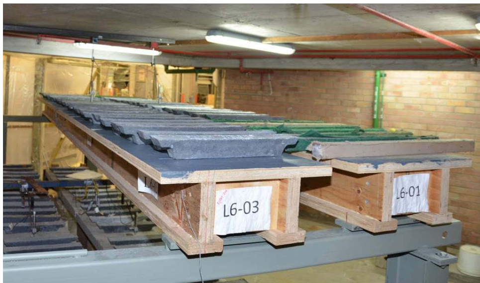
Figure 84: Timber composite beams in humidity chamber
