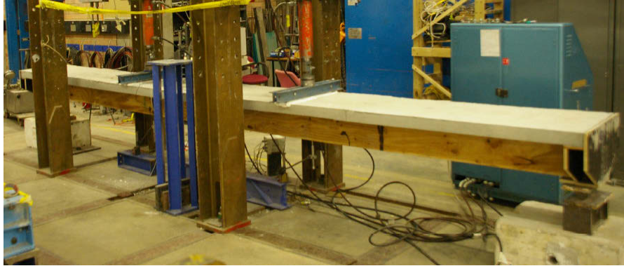
Figure 38: TCC beam under short-term test
