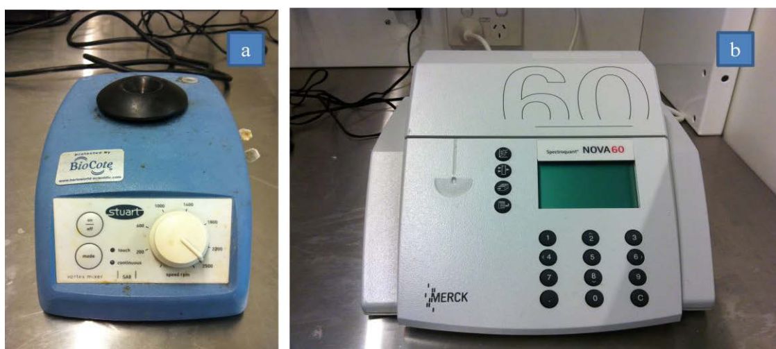
Figure 3.5 Analytical instruments: a) SA7 vortex mixer and b) Spectroquant® NOVA 60, Merck, Germany
