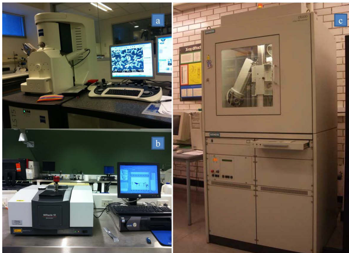
Figure 3.6 Analytical instruments: a) Zeiss Evo LS15 SEM, Germany, b) IRAffinity-1 Fourier Transform Infrared Spectrophotometer, Shimadzu Corporation, Japan, and c) Siemens D5000 X-ray Diffractometer
