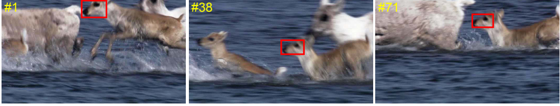
Figure 1.1: An example of online visual object tracking discussed in this thesis. Given a bounding box of an object in the first frame of a video, the task of a tracker is to locate the target in subsequent video frames.
