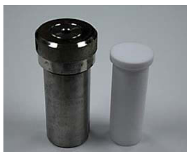
Figure 3.1: Photograph of Teflon Lined Autoclave used as a reactor in hydrothermal growth.
