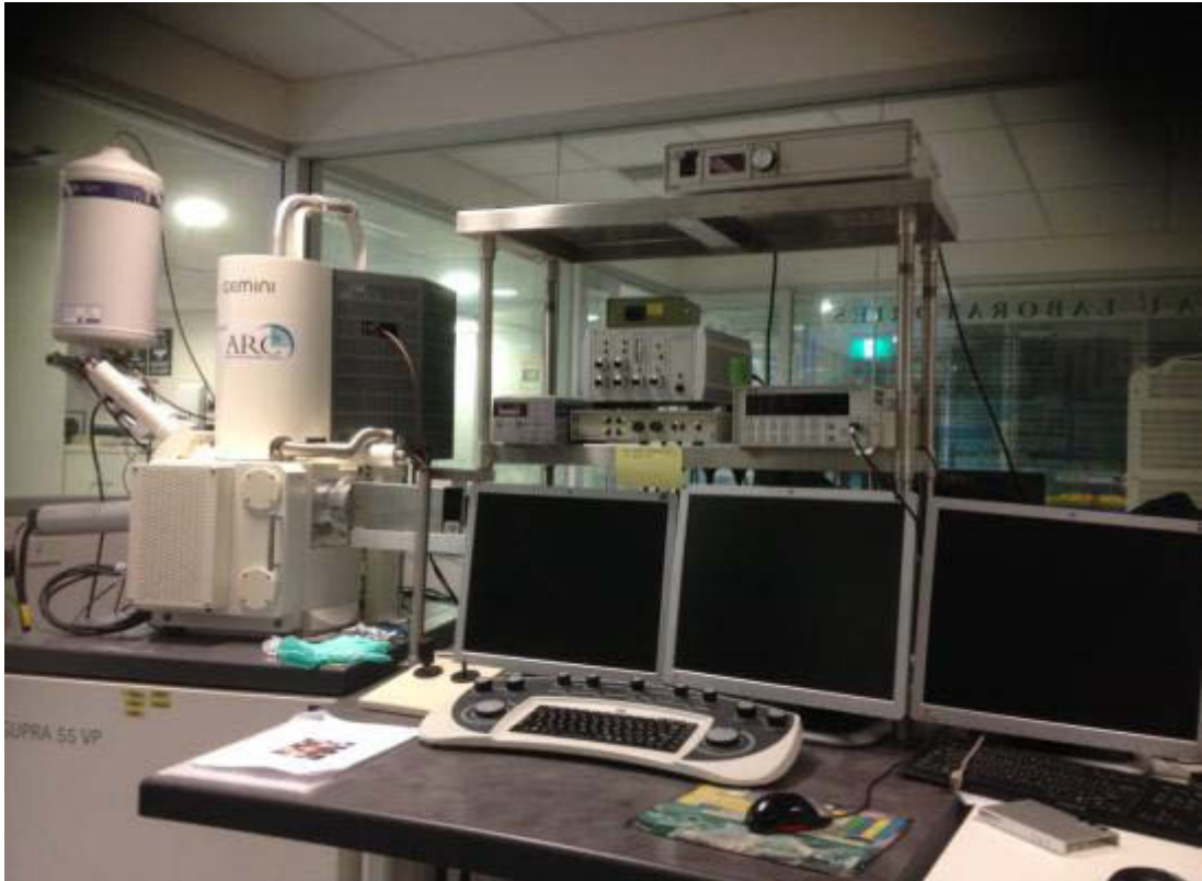
Figure 3.3: High-resolution Schottky field emission scanning electron microscope (SEM Zeiss Supra 55 VP).
