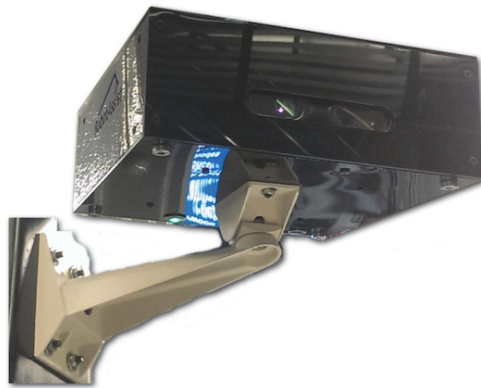
(a) Boxxie – the platform for robust people detection, tracking, and counting in public spaces.
