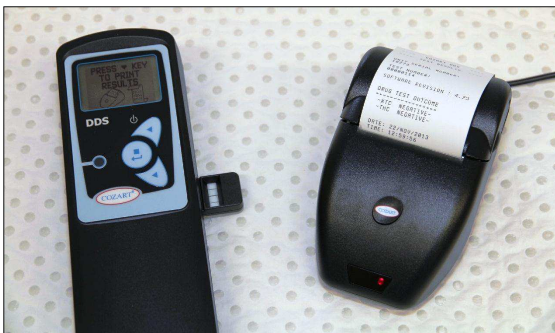
Figure 1-6: The Cozart® DDS digital reader with test cartridge inserted (left) and printer (right).
