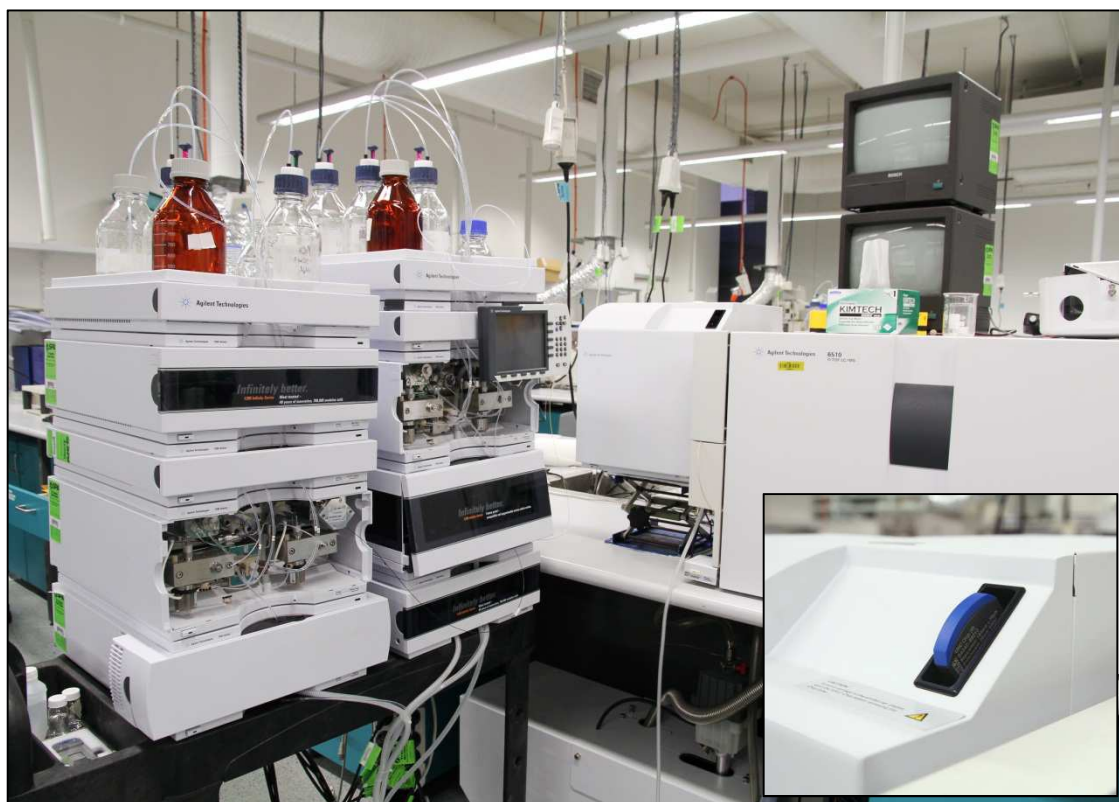
Figure 5-1: Instrument set-up for nano flow LC-chip-Q-TOF-MS and (inset) chip is inserted into slot in chip cube. Sitting on a trolley on the left is the capillary loading pump (also in picture is a DAD and regular LC column compartment not used in these studies). Next to this are the nano pump, autosampler and cooler. Each pump has its own set of mobile phase bottles seen on top of each stack. On the bench is the chip cube mounted on the Q-TOF-MS. A capillary from the autosampler and a capillary from the nano pump connect the LC system to the chip cube.
