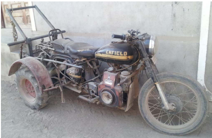
Plate 10: GD's Motorcycle-operated sprayer
