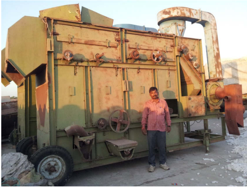
Plate 17: MP's Cotton Stripping Machine
