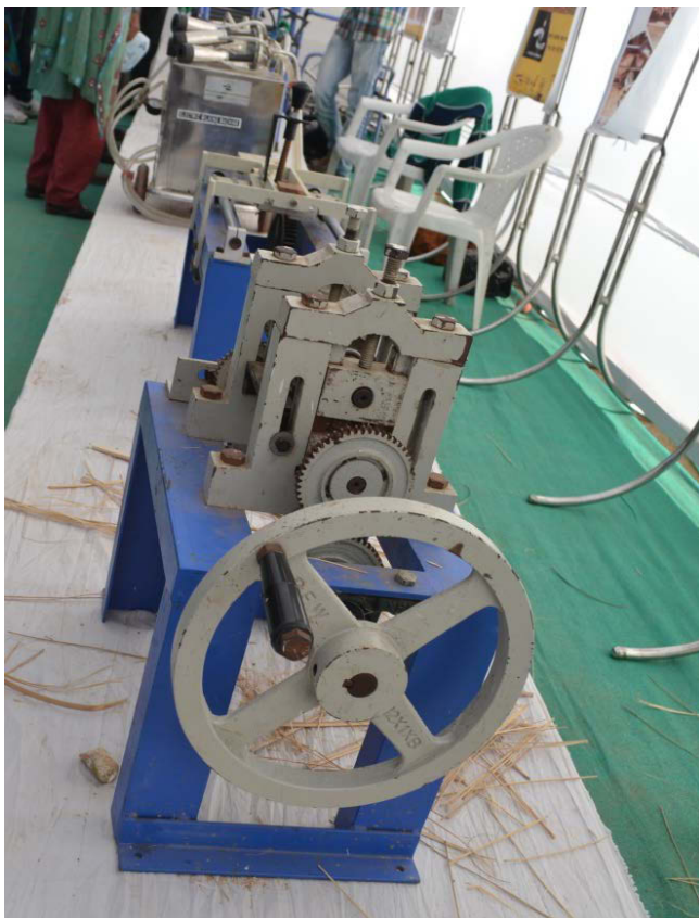
Plate 26 : PP's Bamboo strip and incense stick-making machine
