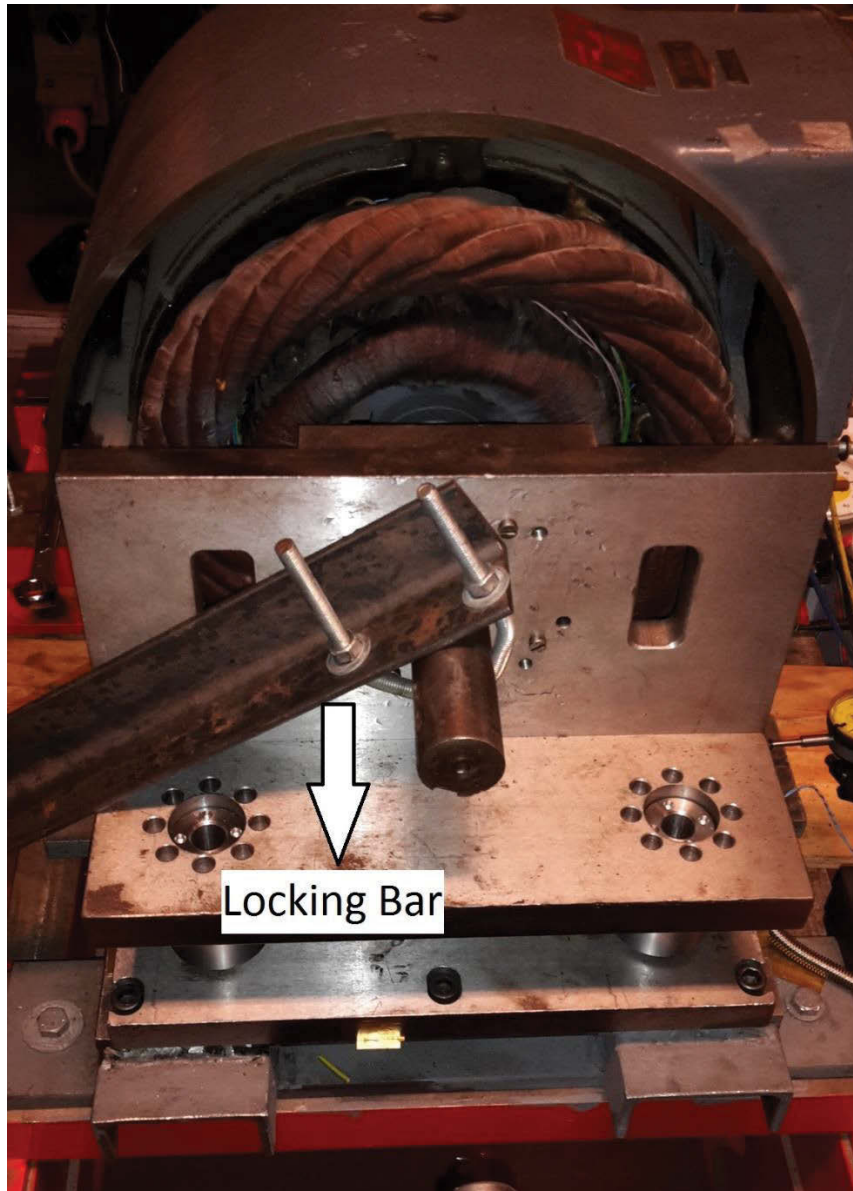
Figure 4.11: rotor with locking bar.
