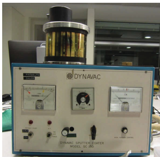
Figure 3.1. DYNAVAC SC150 sputter coater used for Au layer deposition. A Au film with a thickness of \sim 6 nm can be deposited on the substrate by applying the sputter ion source at 100 mA for 30 s.
