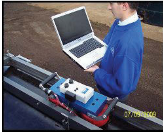
FIGURE 1.1: Industrial MFL tool in operation [1].
