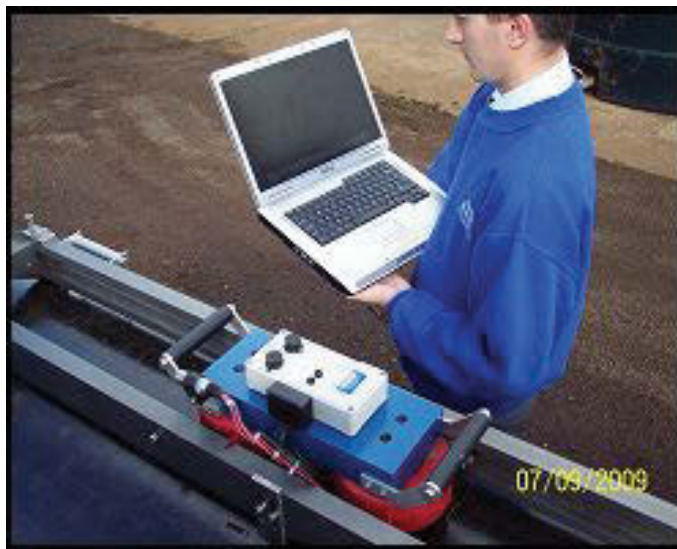
FIGURE 3.18: Industrial MFL tool in use [1]
