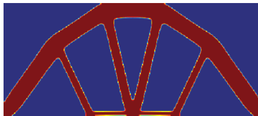
Figure 5-23 Deterministic topology optimization
