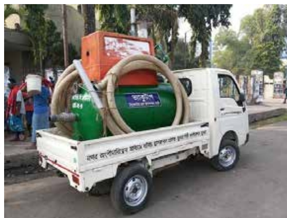
Figure 11 – Retrofitted sludge emptying truck Source: SNV Bangladesh
