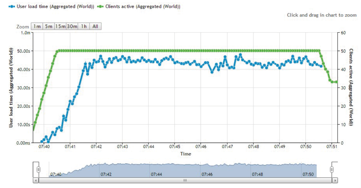
Figure 4.16- Load time vs clients active - 50 virtual users
