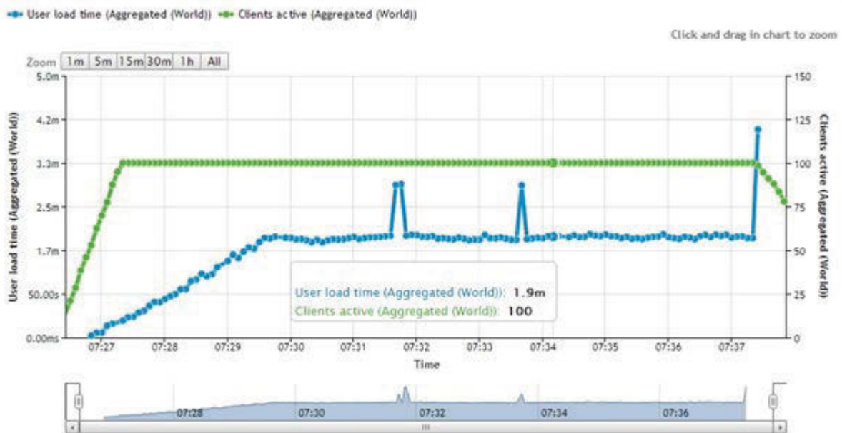
Figure 4.20-Load time vs clients active - 100 virtual users
